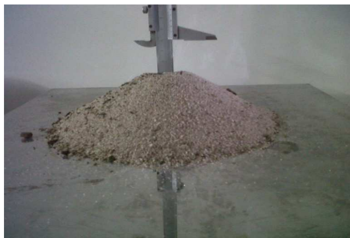
Figure 3-19 Measuring the angle of repose
