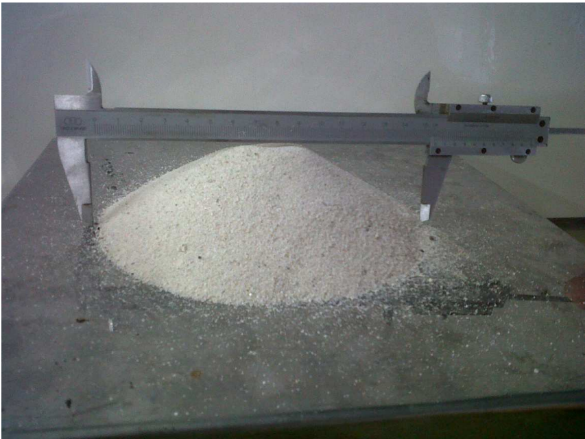
Figure B.9 Width measurement for angle of repose
