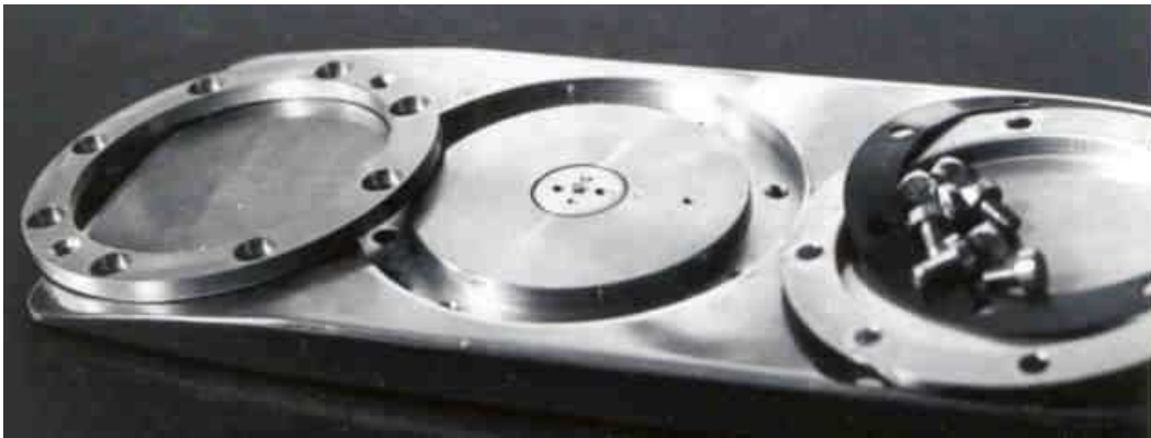
Figure 2-20 (DMT blade components, Marchetti, 2001)
