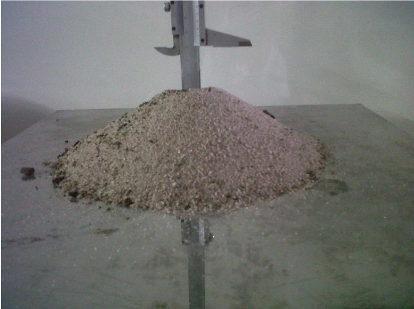
Figure B.8 Height measurement for angle of repose
