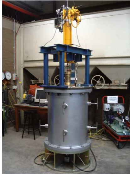
Figure 2-31 Chamber for CPT testing in Sydney (Pournaghiazar et al, 2011)
