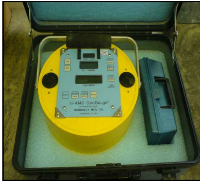
Figure 2-40 Geogauge (CPU Model H4140)
