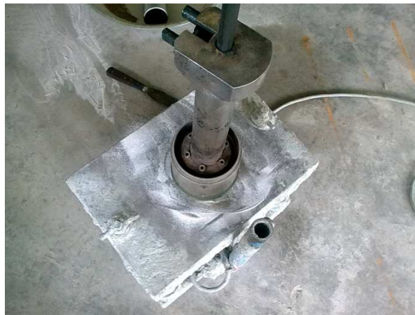
Figure 3-23 Marshall Hammer for compaction assistance
