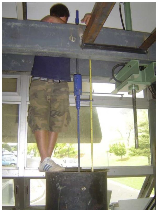
Figure 3-10 DCP Apparatus (CPUT, 2007)
