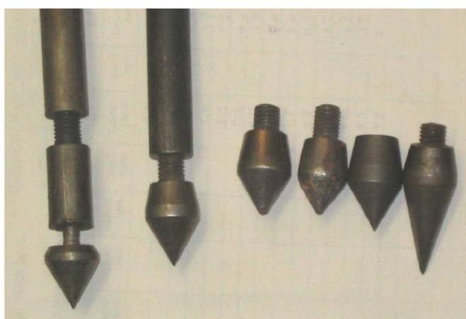
Figure 3-14 Disposable cones for the DCP (Paige-Green, 2009)
