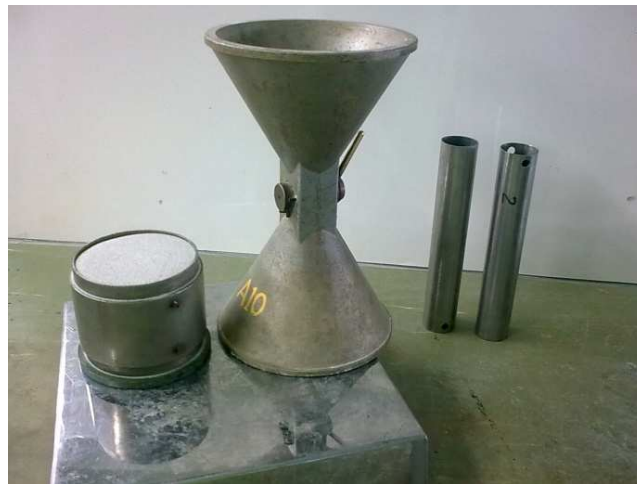
Figure 3-18 Sand replacement cone
