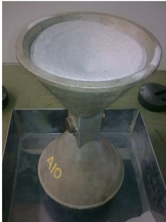
Figure B.10 Apparatus for sand pluviation
