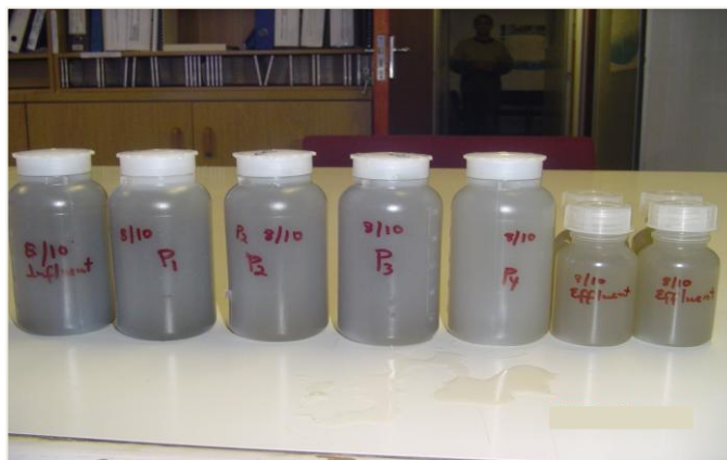
Figure 5-12: Quality of greywater effluent from processes
