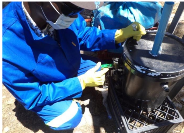
D10: Temperature measurement on the Co-composting process
