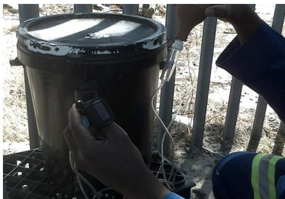
D11: Oxygen meter is used for the measurement of oxygen in the composter
