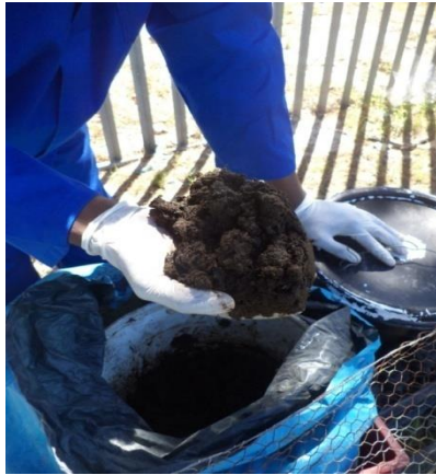
D15: Composted human faeces is taken out from Skyloo composting lab-scale.
