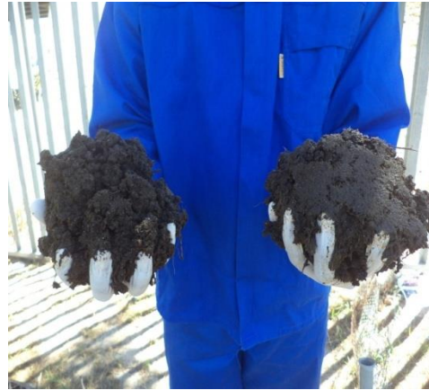
D 14: Three samples of composted faeces are collected from three different lab-scales to measure the moisture content.
