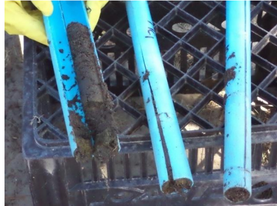
D 14: Three samples of composted faeces are collected from three different lab-scales to measure the moisture content.
