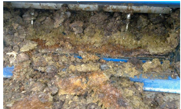
D6: Desiccated HF in the children toilet vaults
