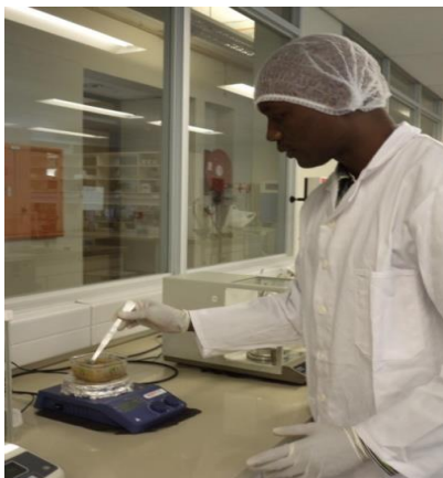
D17: Sample of composted faeces have to be weighed to determine the carbon content.
