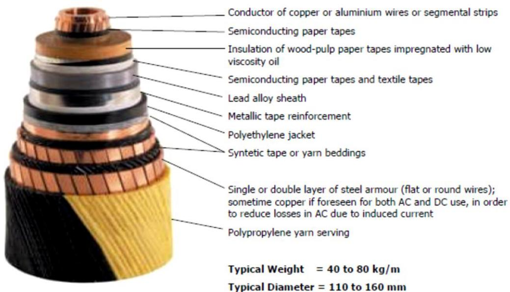
Figure 2.10: Self-contained fluid filled cable (Europacable, 2011)
