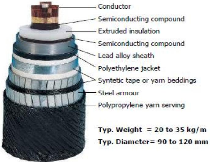
**Figure 2.11: Extruded cable for HVDC applications (Europacable, 2011)**
