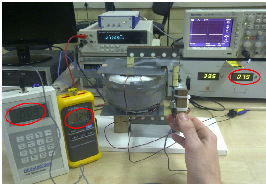
Fig. 3.30 Flux density measured in the air gap of force rig Design 3
