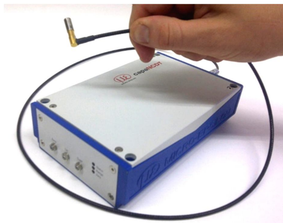
Fig. 3.12 CapaNCDT DT6300 controller with CS02 capacitive displacement sensor
