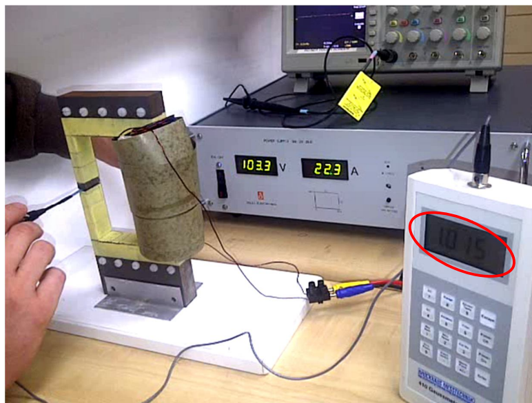
Fig. 3.26 Flux density measured in the air gap of the magnetic circuit for Design 3
