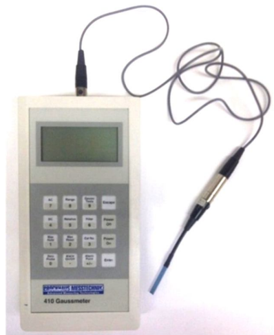
Fig. 3.19 Gaussmeter with transverse Hall probe
