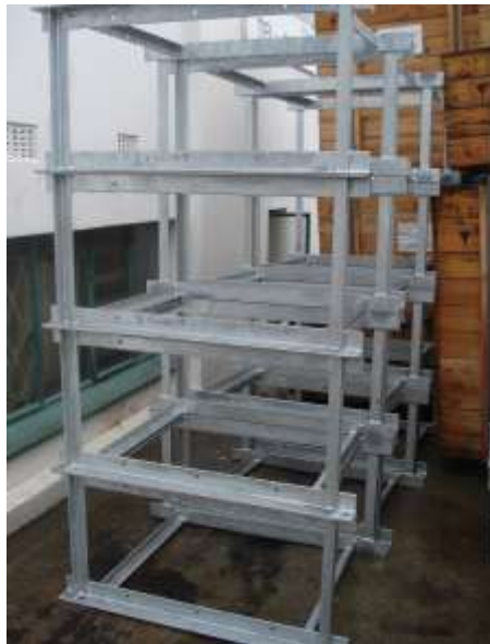
Figure 5.7: Fabricated capacitor rack frame
