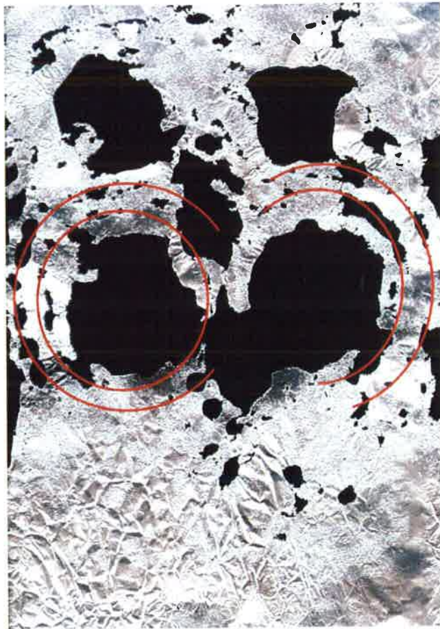
Figure 5-4: The destruction of tinfoil after exposure for 1.5 minutes when the bath was driven by the phase locking system. The average electrical power measured over this test was 70W RMS. Note the large amount of destruction to the upper section of the foil and the four holes showing that four transducers were dissipating most of the electrical power. The relatively undamaged area in the lower portion shows two transducers were not dissipating enough electrical power to cause destruction of the tinfoil
