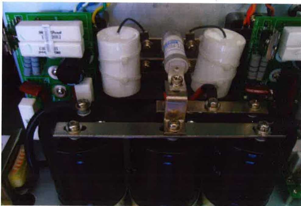
Figure 6.13 Integrated Systems with Dc Bus Capacitors
