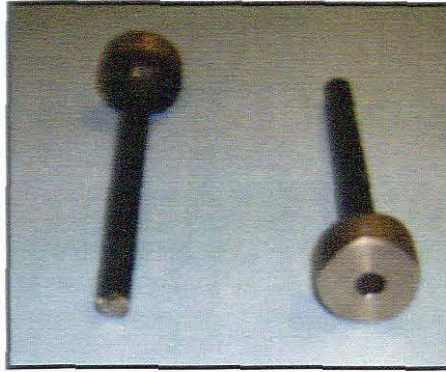
Figure 6.9: The adaptors used to secure the samples for tensile strength tests
