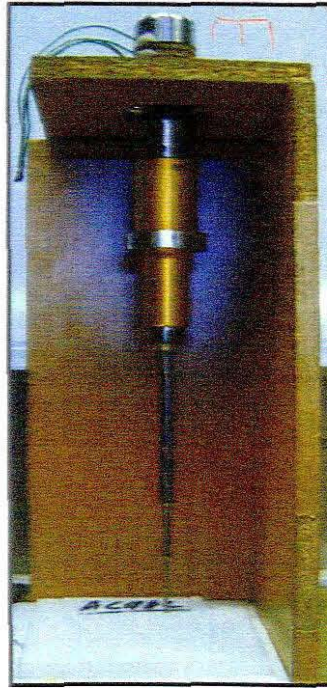
Figure 6.2: Experimental ultrasonic plastic welding setup
