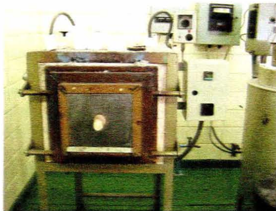
Figure 4.7: The curing oven with electronic temperature controls used for heat experiments
