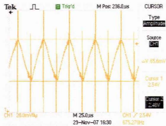
Figure 3.16: An oscilloscope screenshot of the output of the Hall Effect sensor placed at the side of the transceiver coil. The driving pulse frequency and magnitude was 20kHz and 20V p-p respectively
