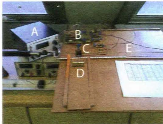
Figure 3.3: The elevated wooden platform situated underneath the transceiver coil. The power supplies and electronic circuitry is indicated by (A) and (B) respectively. The transceiver coil is indicated by (C). The bias magnets and nickel waveguide is indicated by (D) and (E) respectively
