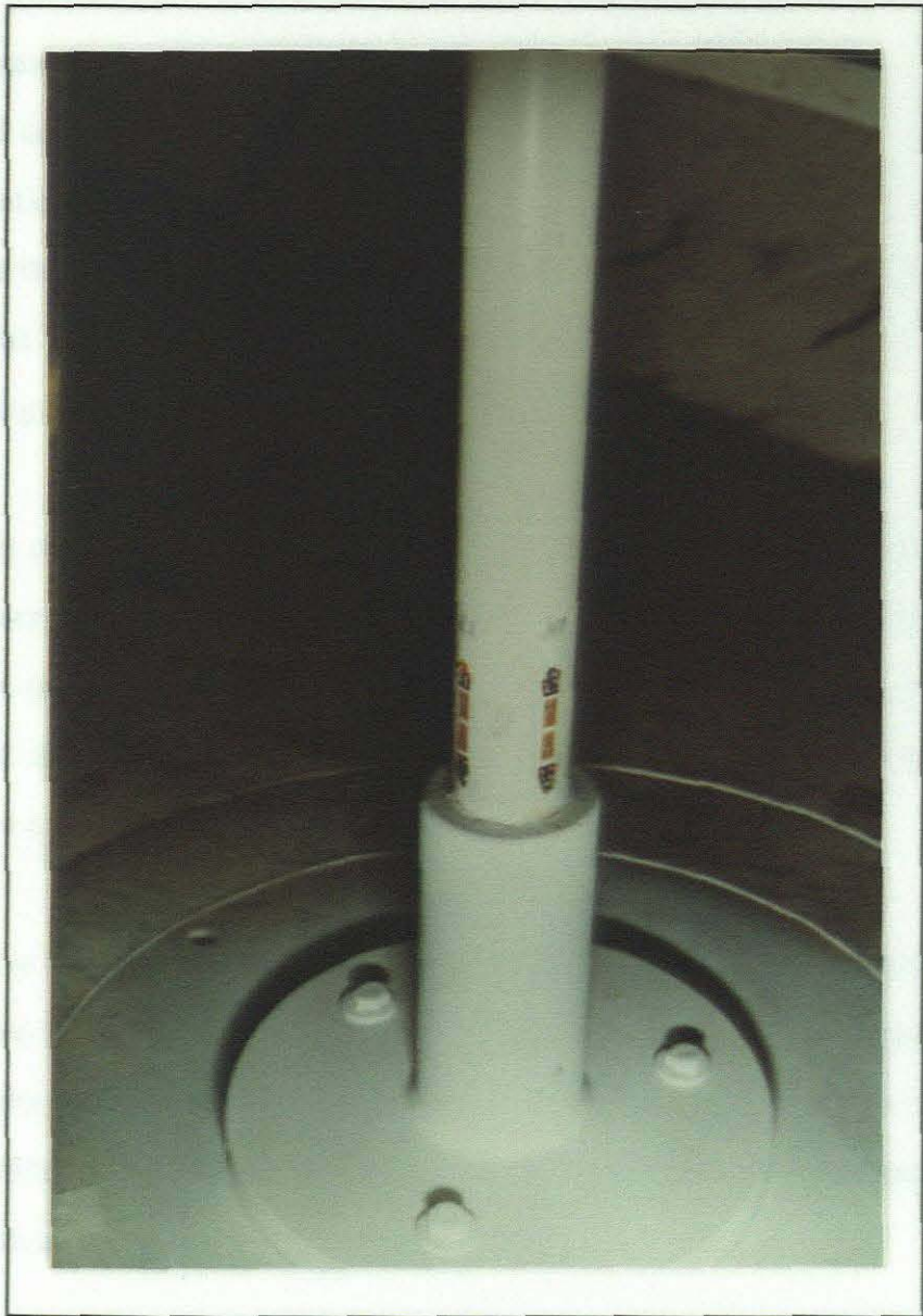
Figure 5.10 : Strain gauge orientation on the circumference of the strain gauge/P.V.C. pipe combination (Photograph 3)
