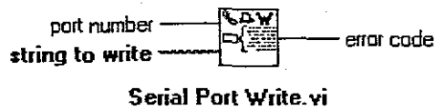
Serial Port Write.vi Writes the data in string to write to the serial port indicated in port number .
