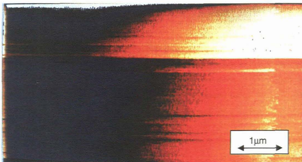
Figure 9.1: STM scan of a gold alloy. The surface is flat and does not show a lot of surface features. A gold alloy surface was chosen because the focus is not on the surface topography but rather in any image artifacts caused by the scanning process. Some features of note in this image are the tip-switch which occurs a third of the way down the image; and the light band on the left hand side. The tip-switch shows where tunneling switched from one protrusion of the tip to another. The light band is a function of insufficient settling time after flyback.
