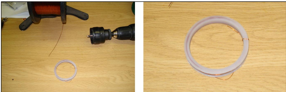
Figure 42: The first stage of the coil prototype manufacture. A nylon inner winding hub was machined to support the 0.5mm diameter coated copper transformer winding wire. The copper wire was wound to 15 turns using a cordless drill
