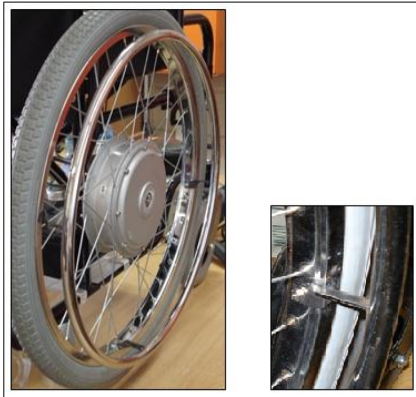
Figure 21: Redesigned pushrim fasteners fixed at 90 degrees to the pushrim, allowing for a greater bending moment
