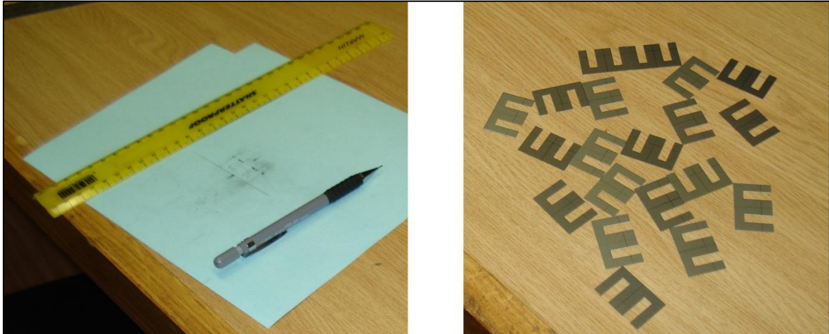
Figure 43: The second stage of the coil prototype manufacture. Standard transformer laminations were manually measured and cut to size using a pair of tin snips
