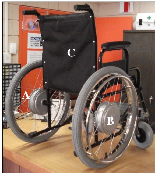
Figure 15: Full Mechanical redesign showing the complete left and right wheel configurations
