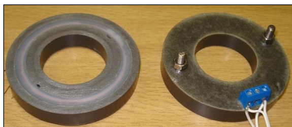
Figure 40: Initial nylon coil with 60 turns cast in the iron filing and polymer mixture
