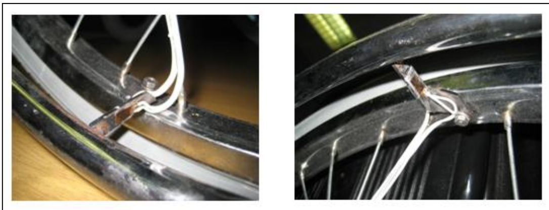
Figure 52: Final prototype strain gauge setup for the user force measurement
