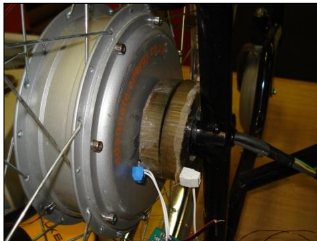
Figure 47: Depicts the final prototype. The primary and secondary transformer generator coils are shown mounted onto the fixed wheelchair frame and moving hub and wheel assembly. The final fixed distance from primary to secondary coils was 1mm
