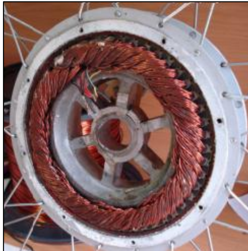
Figure 13: Internal structure of the 400 series hub motor
