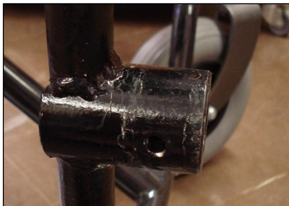
Figure 11: Final machined hub fixed to the wheelchair frame
