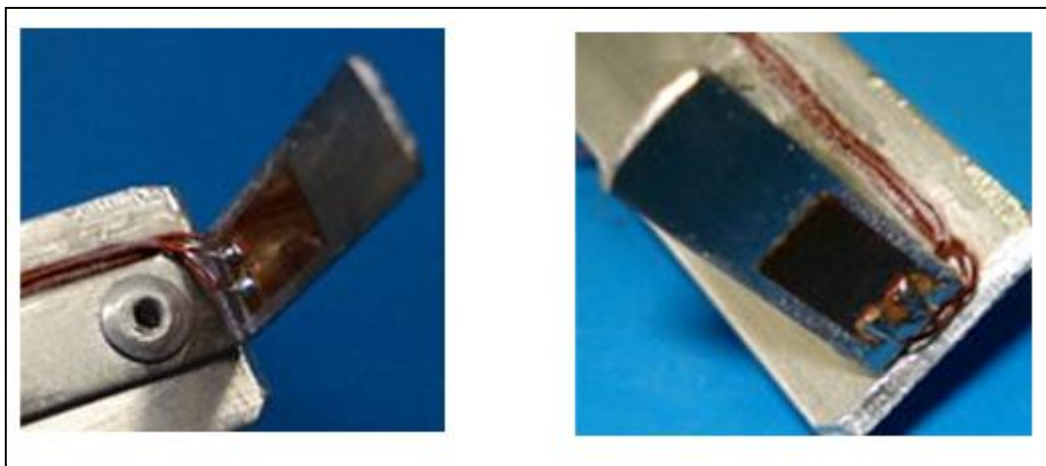
Figure 29: Prototype joystick assemblies constructed out of spring steel while mounted on aluminium angle iron
