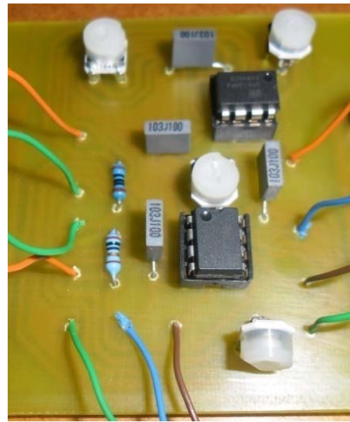
Figure G.3: The fabricated preamplifier circuit with the (a) OPA657 op-amp and (b) TL702 and AD627 op-amps
