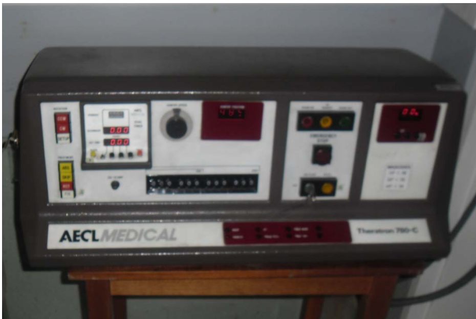
Figure G.15: The ADCL Medical Theratron 780-C control panel
