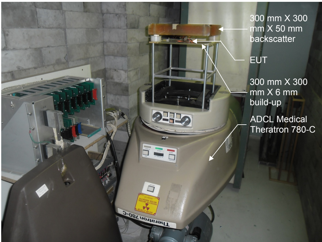
Figure G.12: The ADCL Medical Theratron 780-C with the SQUID sensor on the build-up
