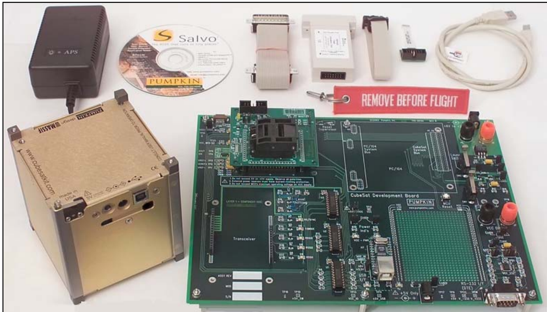
Figure 2.4: CubeSat Kit by Pumpkin (Adapted from Pumpkin, 2003)
