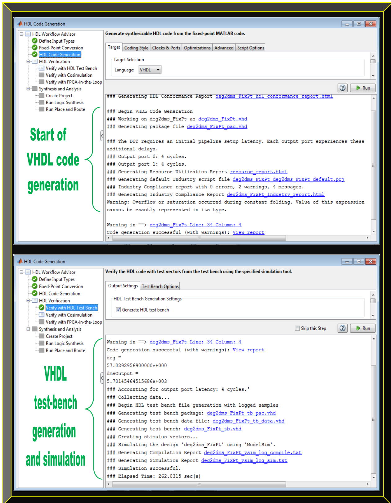
Figure 5.24: deg2dms.m conversion to VHDL and the algorithm verification processes
