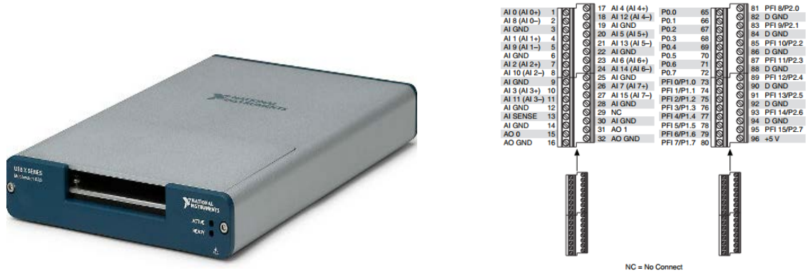
Figure 4.4: The block and pin diagram for the NI 6343 DAQ card (National Instruments, 2014)
