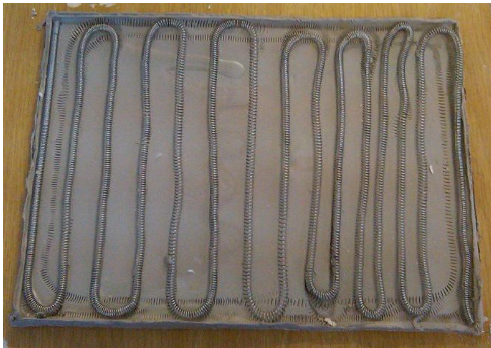
Figure 5.6: Actual photo of heating element on the top part
