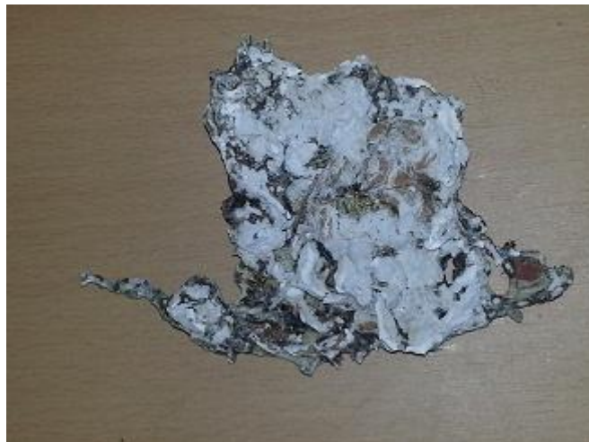
Figure 6.22: HDPE sample before gasification
