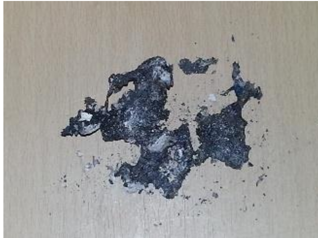
Figure 6.21: LDPE sample after gasification
