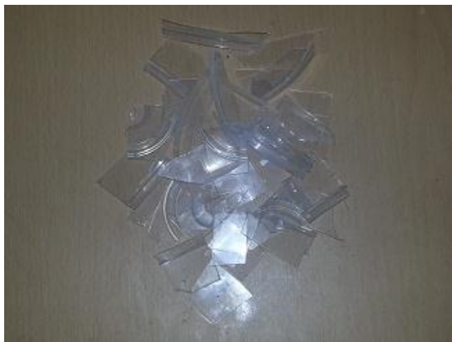
Figure 6.20: PP sample before gasification
