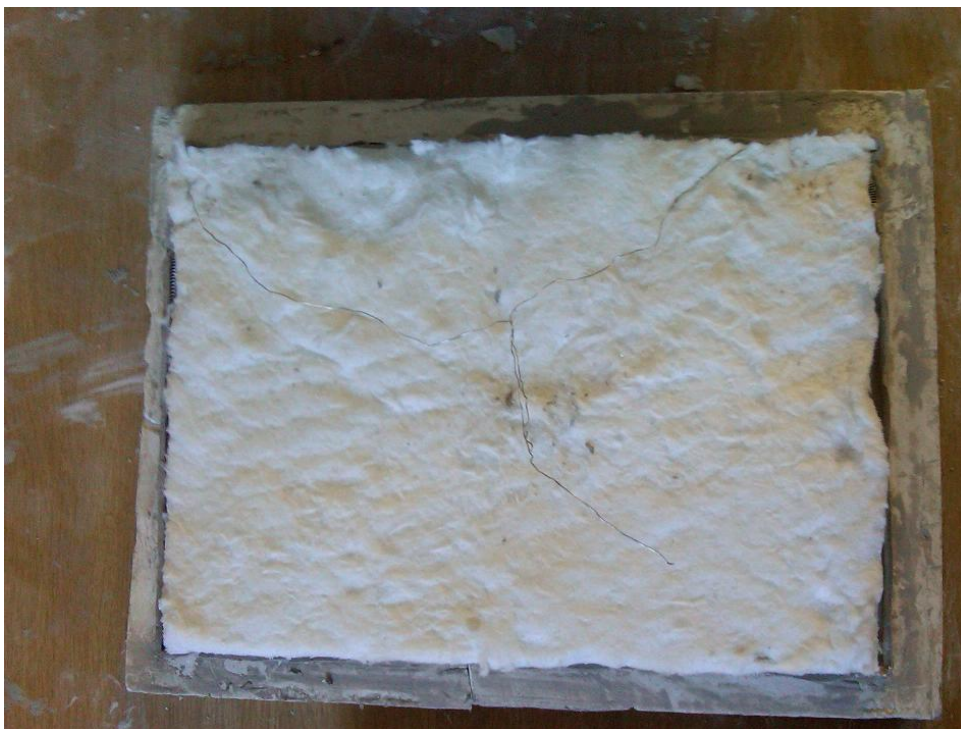
Figure 5.8: Actual photo of the fibre blanket covering the heating element
