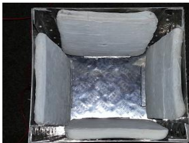
Figure 5.20: Top view of gasifier with heaters
