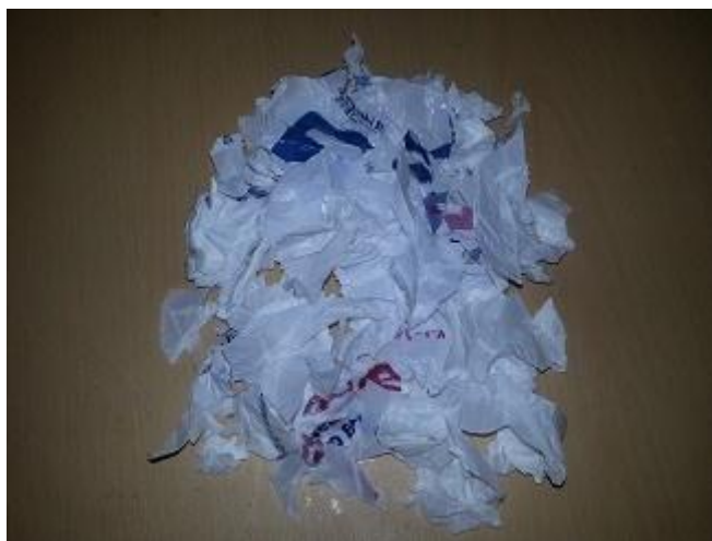
Figure 6.17: HDPE sample before gasification
