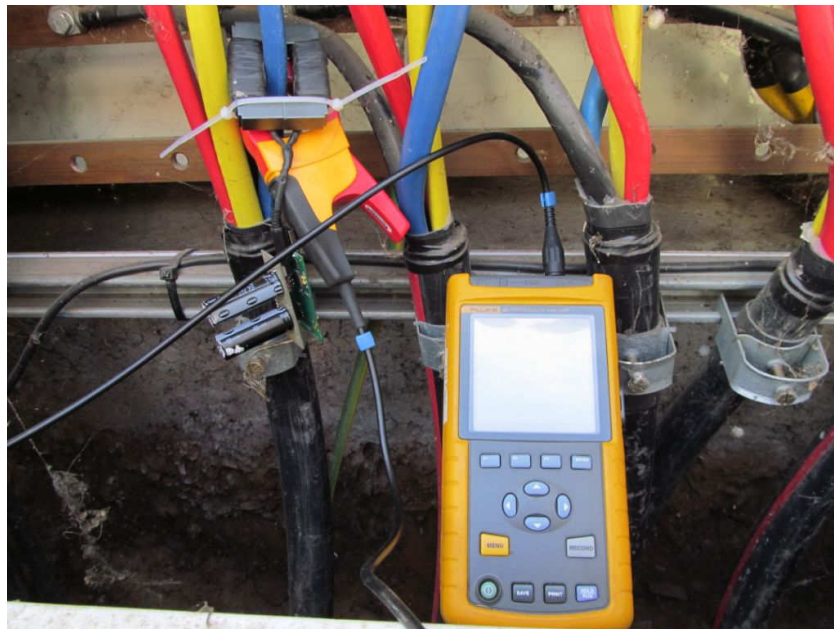
Figure 6-3 Close-up of current monitoring devices on blue phase feeding Mash Street
