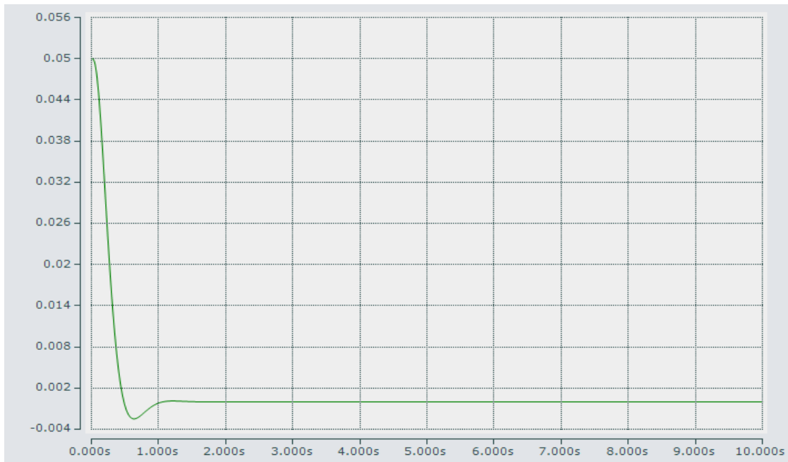
Figure 8.20: Position of the magnetic levitation system when the set-point is y^{sp1}=0[m]
