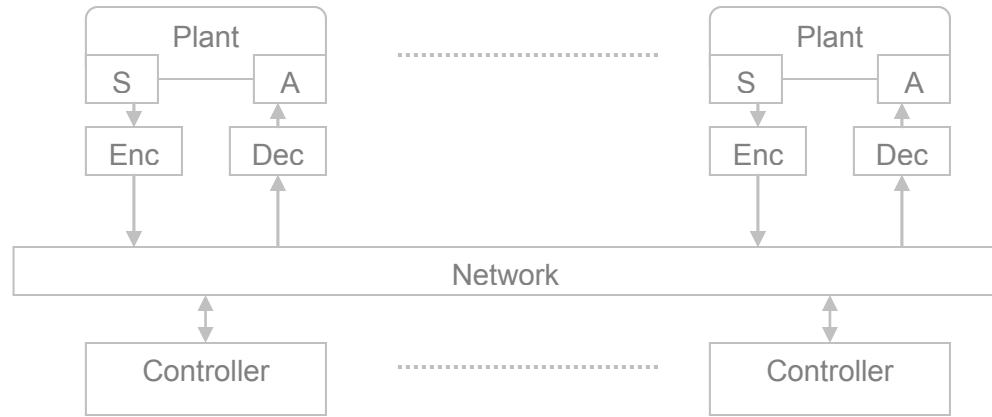
Figure 1.3: Typical Network Control System architecture In this architecture the network is considered explicitly as part of the control system, where S = Sensor, A = Actuator, Enc = Encoder, Dec = Decoder
