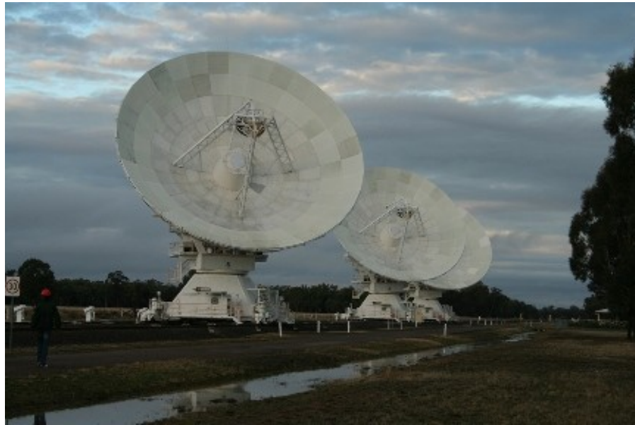
Figure 3.3: Interferometer Array ATNF, Narrabri, Australia 2006, 22m dish diameter in a 6 dish array.
