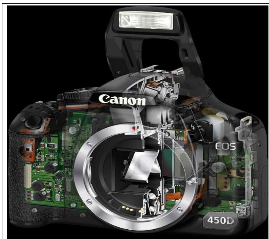
Figure 2.4: Display the internal structure of a camera
