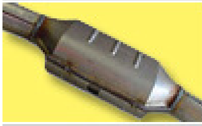
Figure 2.3 A completed under floor catalytic converter as part of the exhaust system. (Source: Anonymous 6, 2009: Online )
