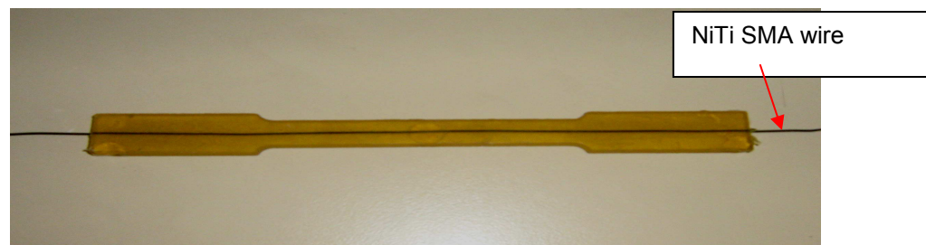
Figure 6.12: Dog bone NiTi SMA/polyurethane specimen (single wire)
