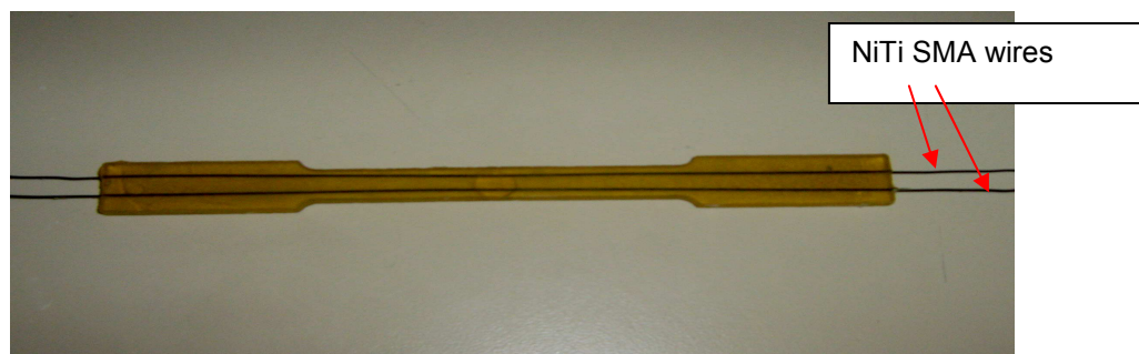
Figure 6.13: Dog bone NiTi SMA/polyurethane specimen (double wire)
