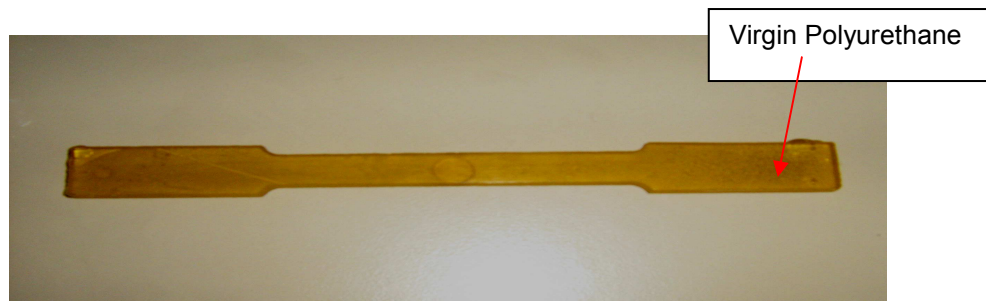
Figure 6.11: Dog bone virgin polyurethane tensile test specimen
