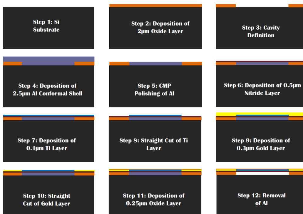
Figure 4-3: Metal bolometer virtual fabrication used CoventorWare
