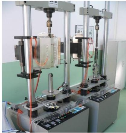
**Figure 5.12:** Creep machine W+b (Wolter + Bai) LFM2 =30kN.
