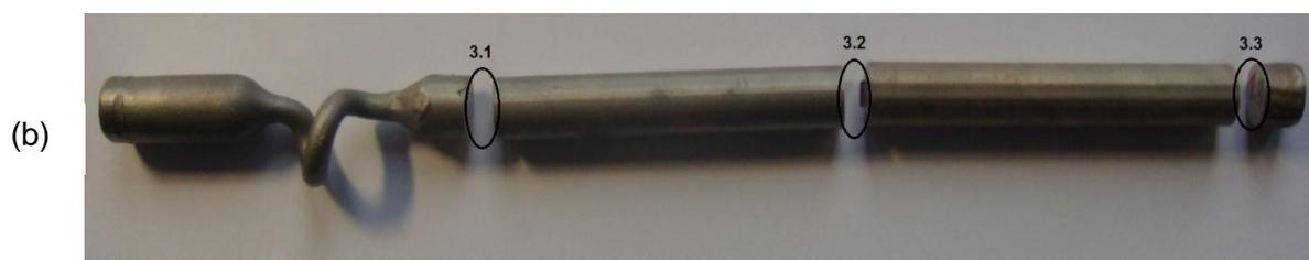
**Figure 6.2:** a) Cutoff machine for samples b) Cross sections samples for rod 3.
