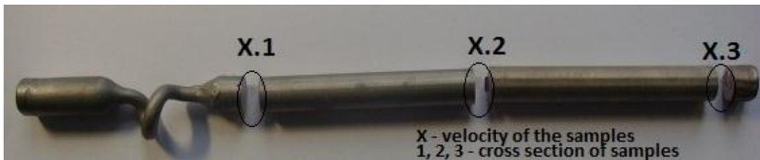
**Figure 5.4:** Cross sections of casting rod 3 mm/min.
