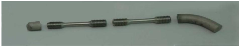
**Figure 5.11:** Samples for creep test
