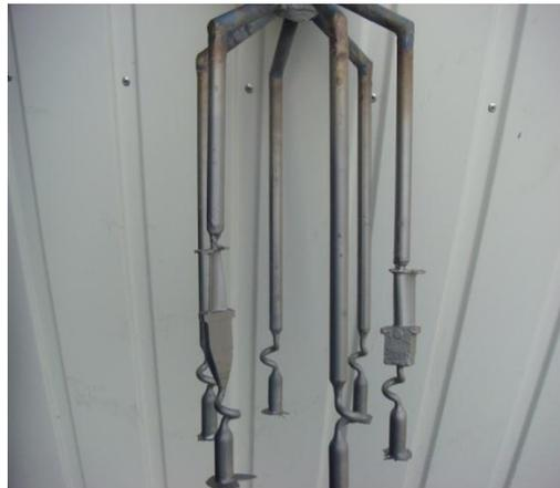
**Figure 4.7:** The casting assembly after removal of the ceramic shell and sandblasting.
