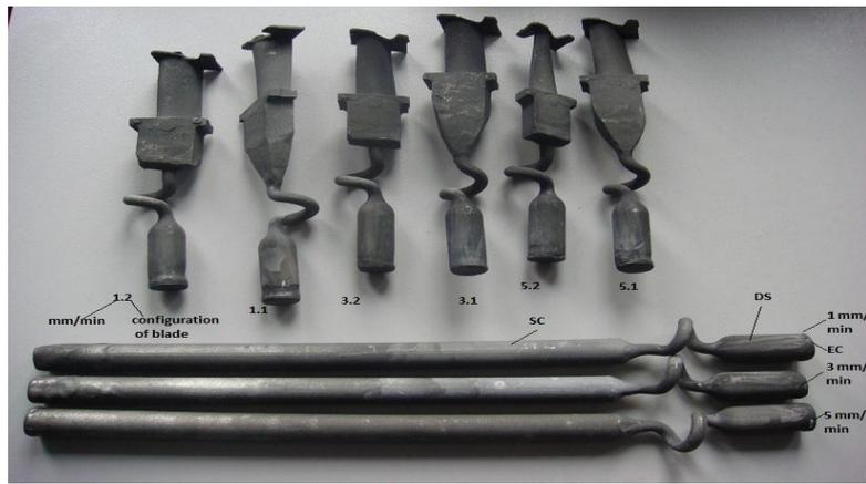
**Figure 6.19:** Macrostructural analysis for turbine blades and casting rods at velocity 1; 3; 5 mm/min.
