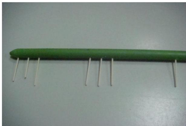
**Figure 4.5:** Thermocouples in wax pattern bar to identify temperature distribution at different withdrawal rates of solidification process.
