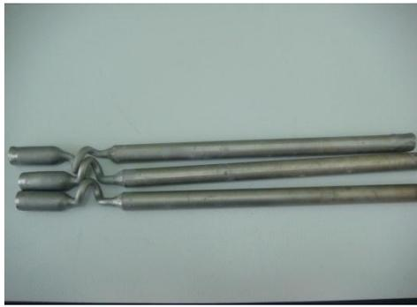
**Figure 6.1:** Casting rods for different withdrawal velocities for preparing samples.
