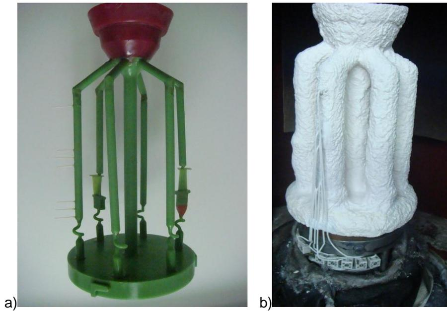
**Figure 4.6:** a) Wax pattern of turbine blade and castings rods; b) ceramic shell mould with thermocouples connected to ALD machine.
