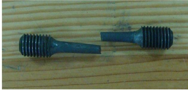
**Figure 5.13:** Sample after creep test.
