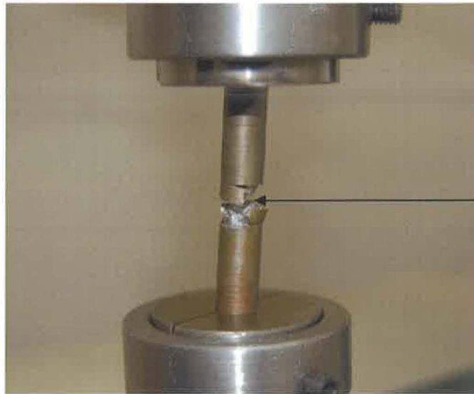
Figure 5.3: Photograph of the fractured un-heat-treated welded specimen
