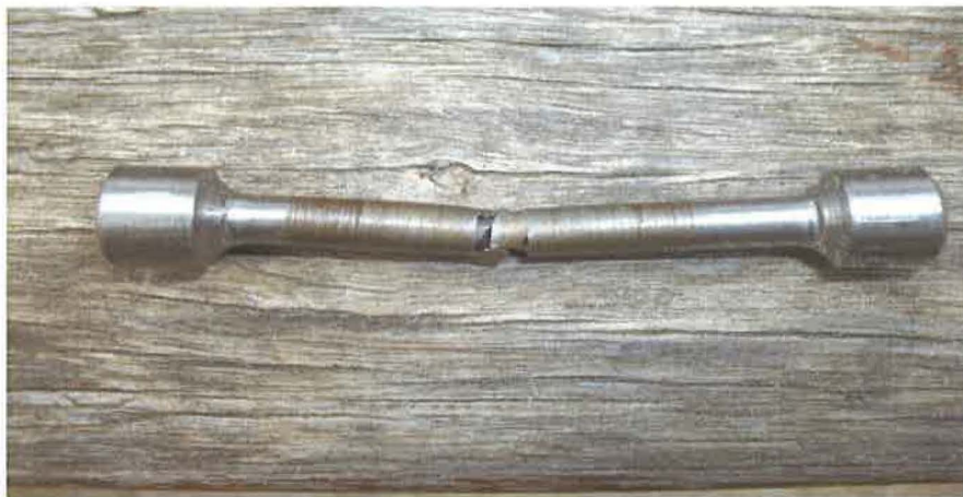
Figure 5.1: Photographs and the sketch of the preparation of the welded specimen for the tensile tests.
