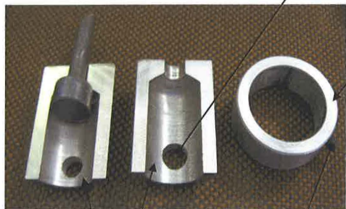
Bushes to hold the specimen
