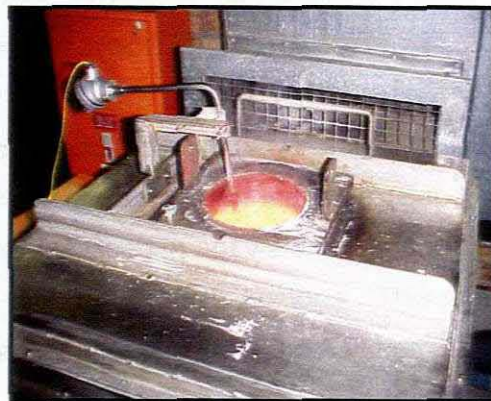
Figure 5.7: Temperature monitoring thermocouple. Note: bath is in operation
