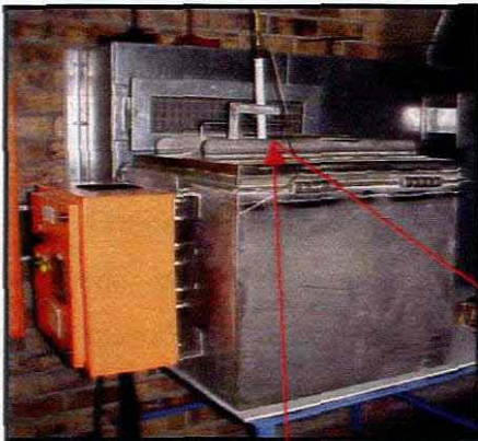
Figure 5.1: Salt bath furnace
