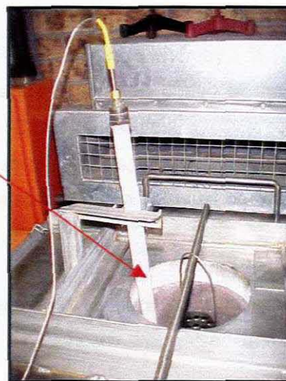
Figure 5.3: Temperature monitoring thermocouple
