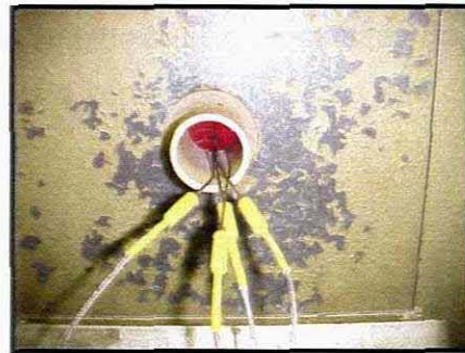
Figure 4.13: Temperature monitoring thermocouples
