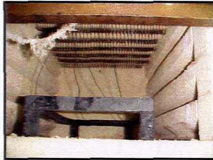
Figure 4.11: New elements on top surface
