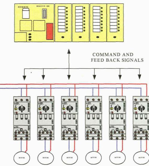
Above the links from the PLC to the compact motor starters(switch gear) can be seen. The interface to the switch gear will be by means of potential free contacts.
