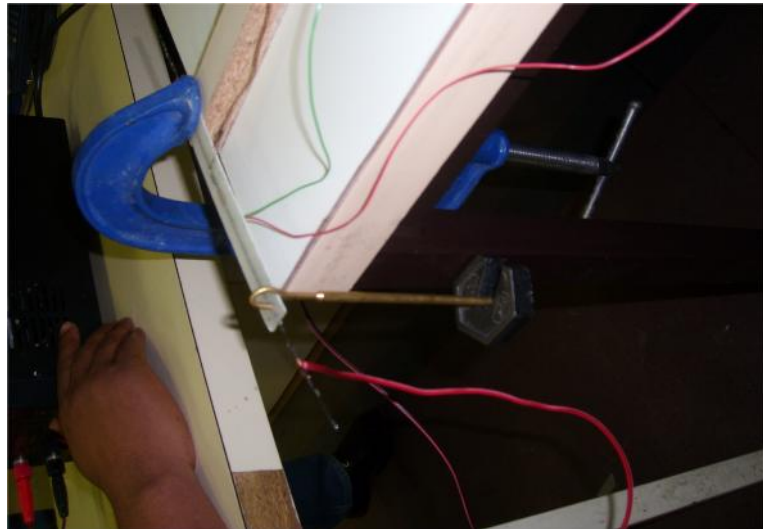
Figure 12: Testing of 1 pre-strained embedded NiTi wire
