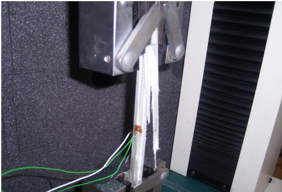
Figure 3.6: Test specimen secured in the tensile machine's jaws
