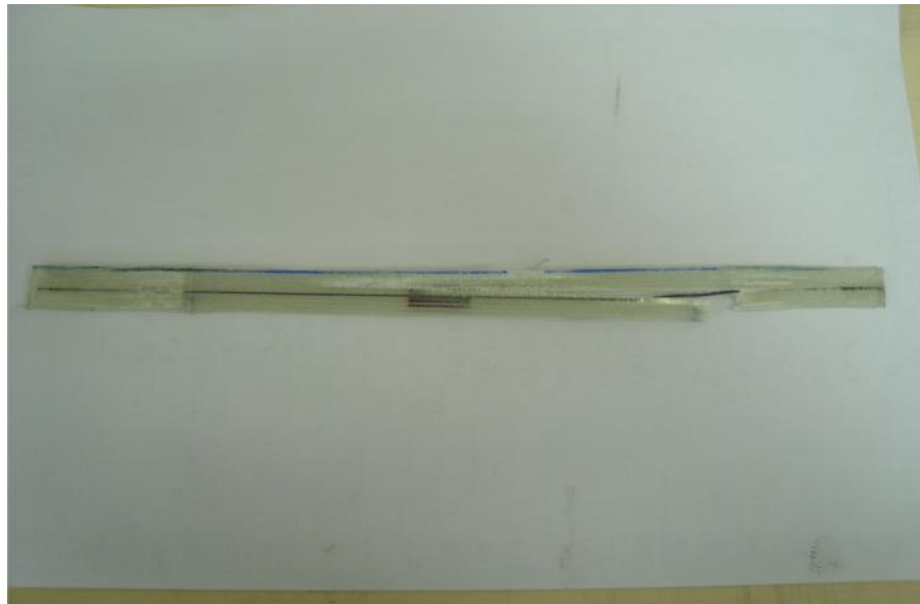
Figure 7.6: Tensile failure mode of the specimen with 1 embedded NiTi alloy wire
