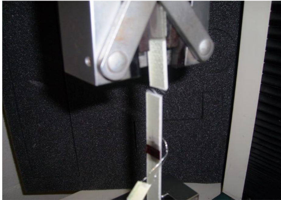
Figure 3.15: [90°] tensile test specimen failure
