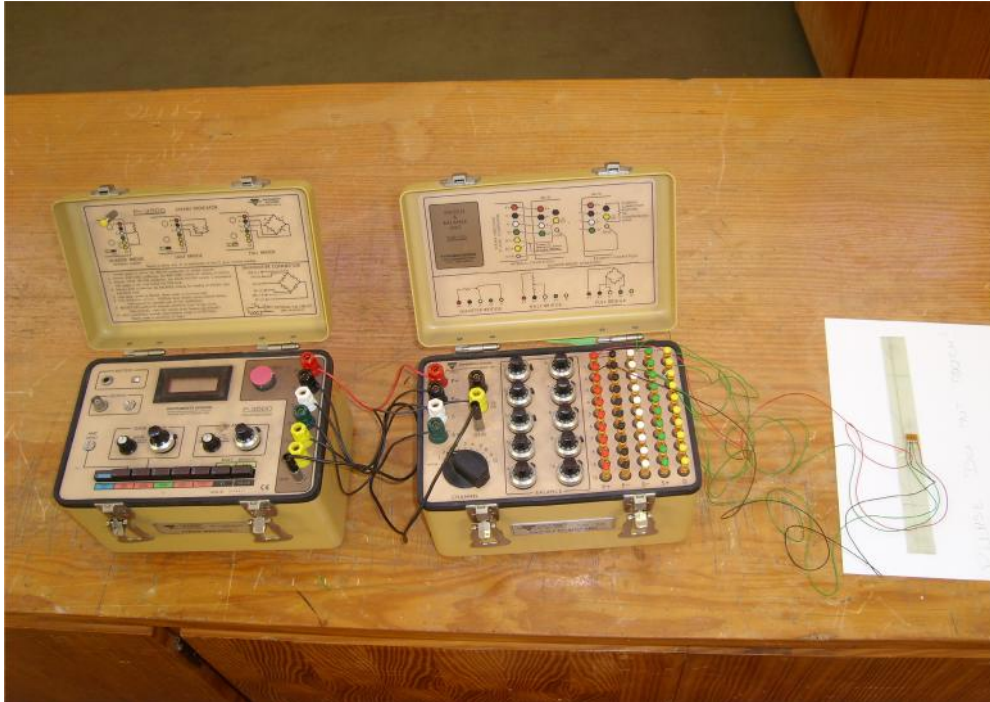
Figure 3.5: A quarter bridge strain gauge connection
