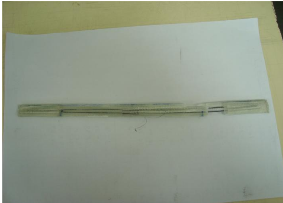
Figure 7.7: Tensile failure mode of 2 embedded NiTi wires in the composite specimen
