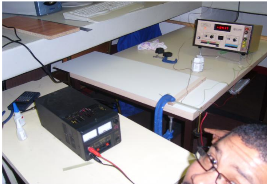
Figure 7.11: An experimental setup for heating an embedded pre strained NiTi alloy wires
