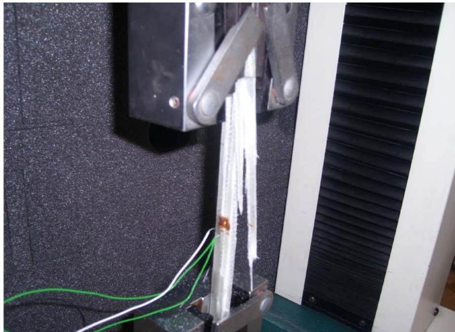
Figure 3.12: [0^\circ] tensile test specimen failure.
