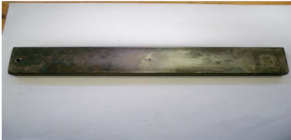
Figure 4.12. Specimen surface heated to dull orange colour with oxy-acetylene flame and quenched in water
