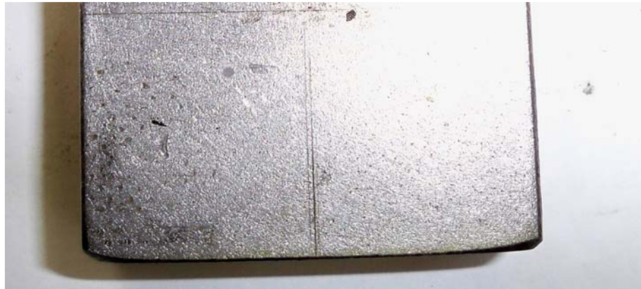
Figure 4.10. Specimen surface impacted with the tips of bristles of a wire brush
