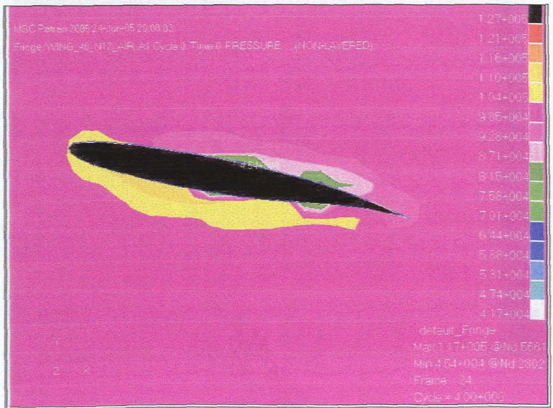
The pressure distribution for Boeing F airfoil. (AOA equal to 12)
