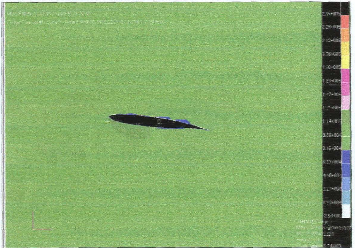
The pressure distribution for Boeing F airfoil. (AOA equal to 8)
