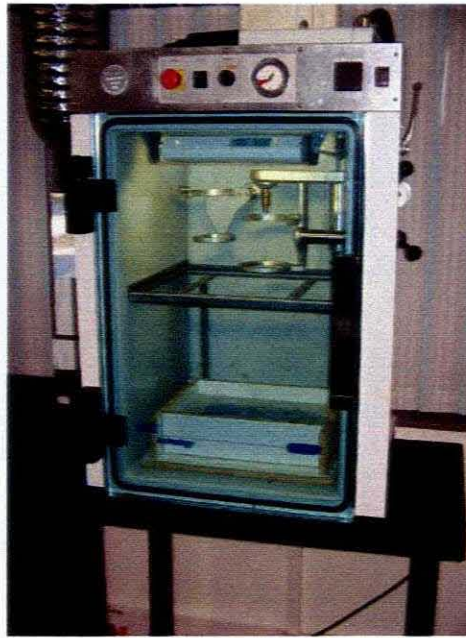
Figure 3.12: Vacuum chamber with silicone mould
