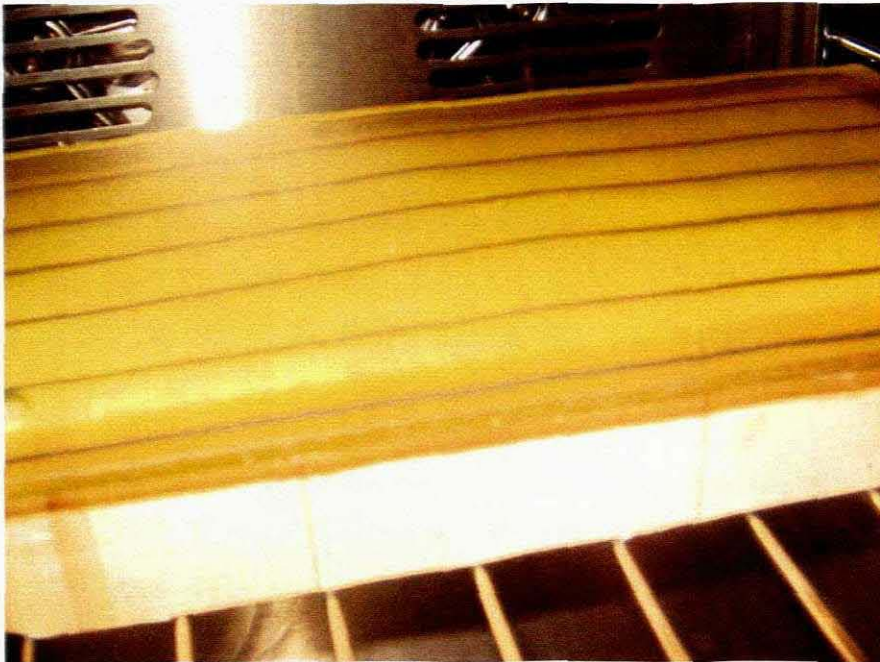
Figure 4.19: The SMAHC plate bulging (negative curvature).
