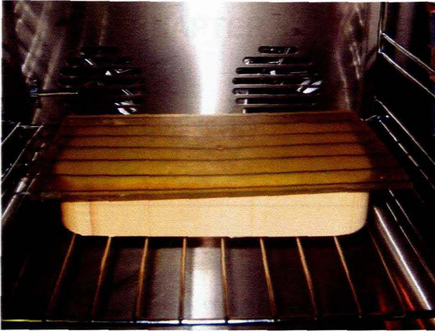
Figure 4.20: End of experiment showing very slight positive curvature.
