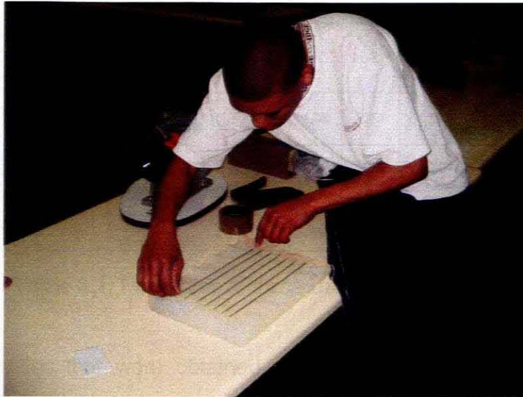
Figure 3.14: Lacing/Embedding SMA wires into mould-base
