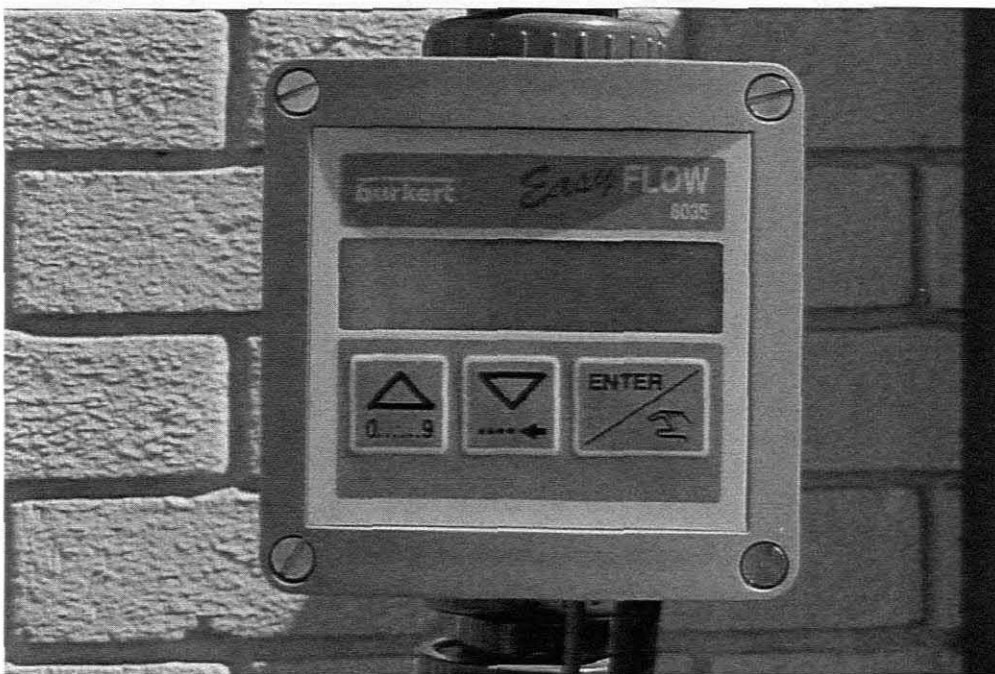
Figure 3.6: Digital flow transmitter
