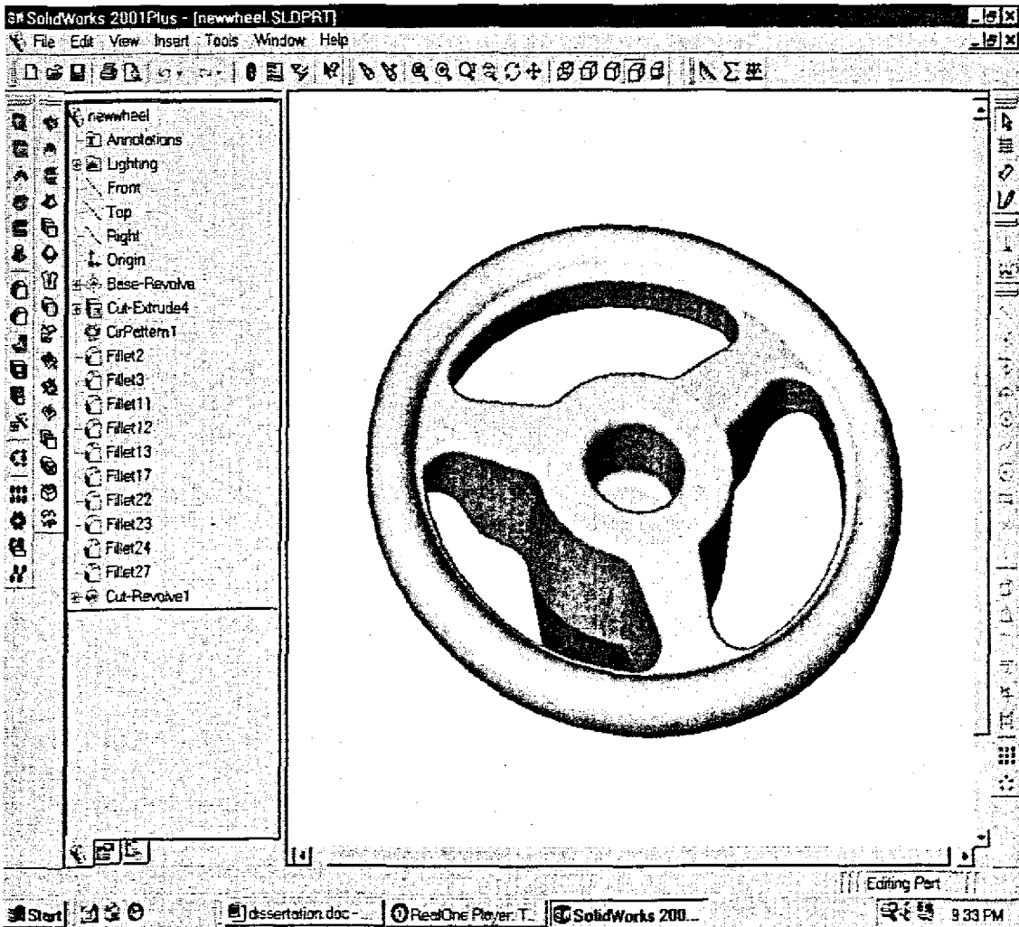
Figure 7.4. Steering wheel, front-side view in SolidWorks (Compliments of Atlas Plastics)
