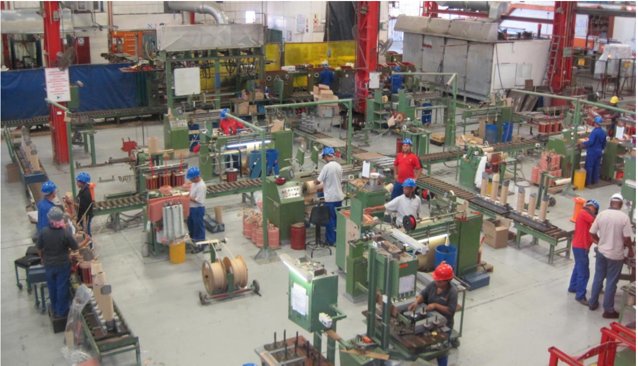
Figure 5.4: New U-shaped roller conveyors after lean change
