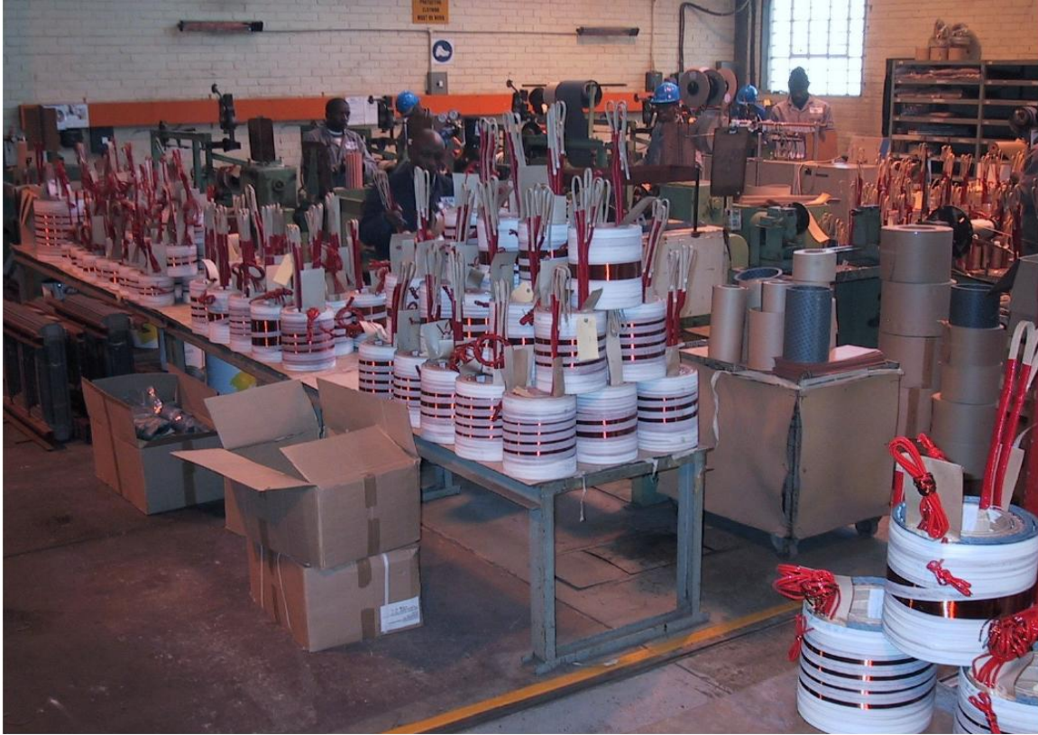
Figure 5.1: Poor house keeping before lean change
