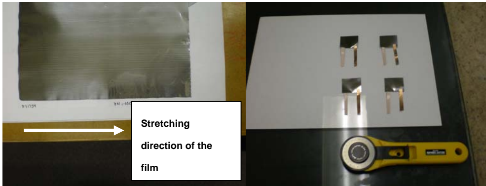
Fig 5.1: Sensor from PVDF film
