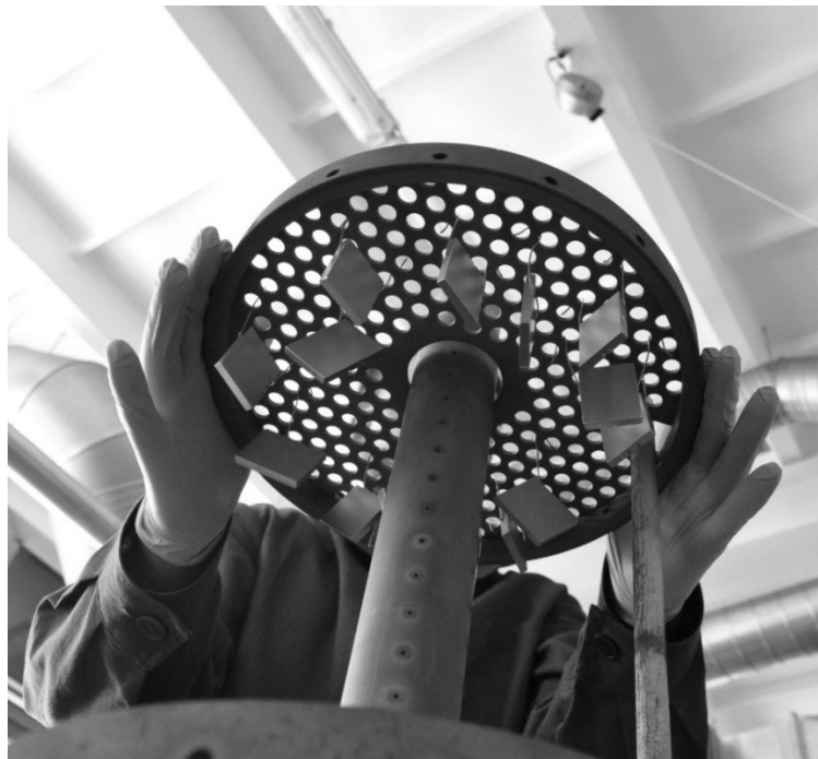
Figure 39. Inconel 617 samples being loaded into CVD process chamber for coating (photographed by Slawomir Kotowski, 2014).
