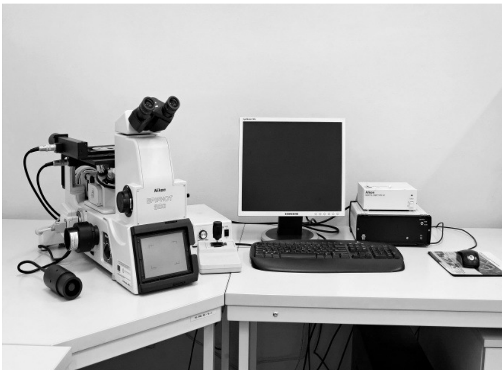
Figure 12 Metallurgical microscope Nikon EIPHOT 300 for observation of coating microstructure (Research and Development Laboratory for Aerospace Materials, 2014).
