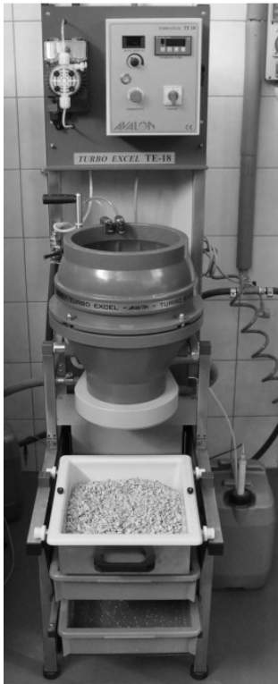
Figure 38(a). Avalon TE-18 centrifugal tumbler and (b) process chamber during polishing of Inconel617 sheets.
