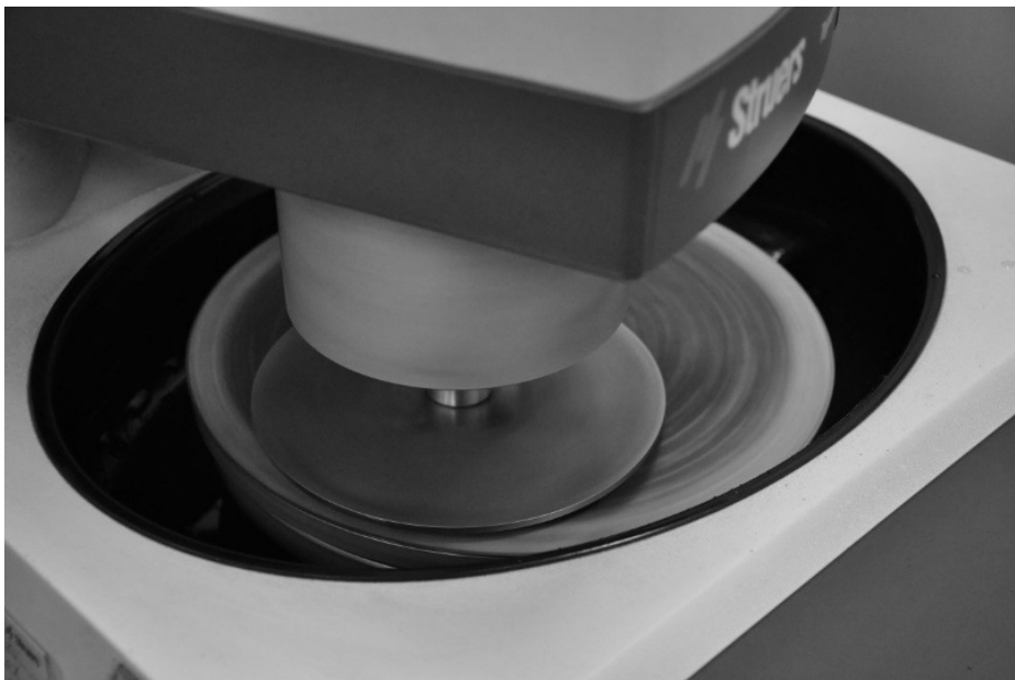
Figure 15. Variable speed grinding/polishing machines Struers TegraPol-25 + TegraForce-5 + TegraDoser-5 (Research and Development Laboratory for Aerospace Materials, photographed by Slawomir Kotowski, 2014).
