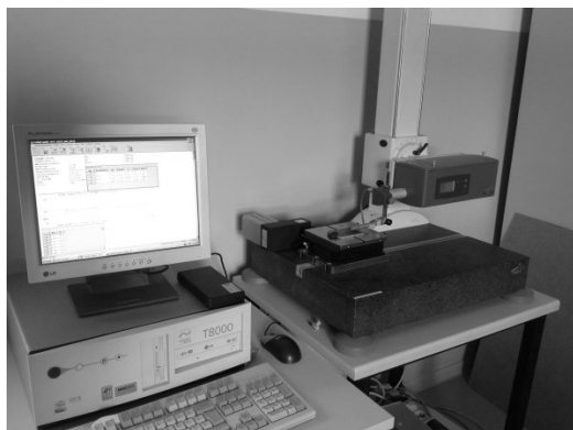
Figure 20 (a) HOMMEL T8000 roughness and contour measuring system and (b) the device probe during roughness measurement (Research and Development Laboratory for Aerospace Materials, photographed by Slawomir Kotowski, 2014).
