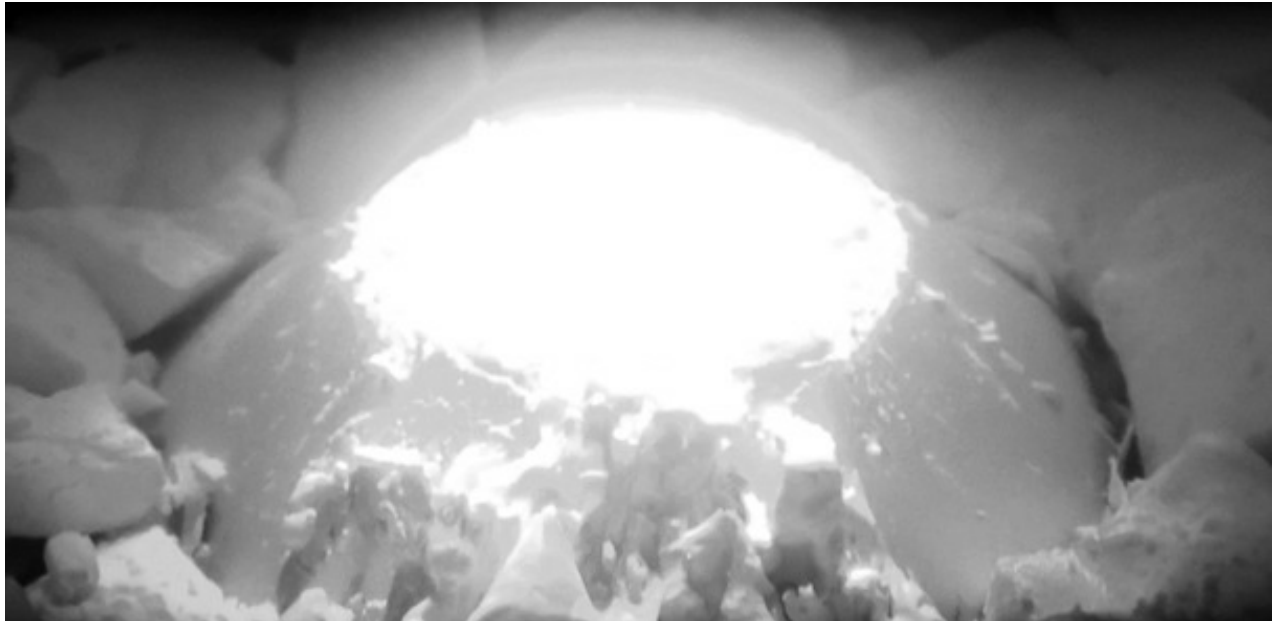
Figure 31 10% YPSZ ingot being melted by electron beam during the experiments discussed in this report (photographed by Slawomir Kotowski, 2014).
