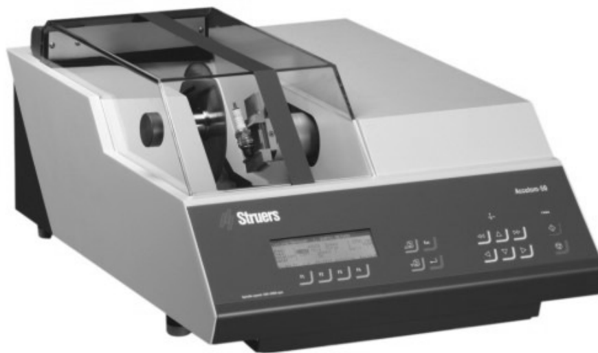
Figure 13. Struers Accutom-50 precision cutting machine (Research and Development Laboratory for Aerospace Materials, photographed by Slawomir Kotowski, 2014).
