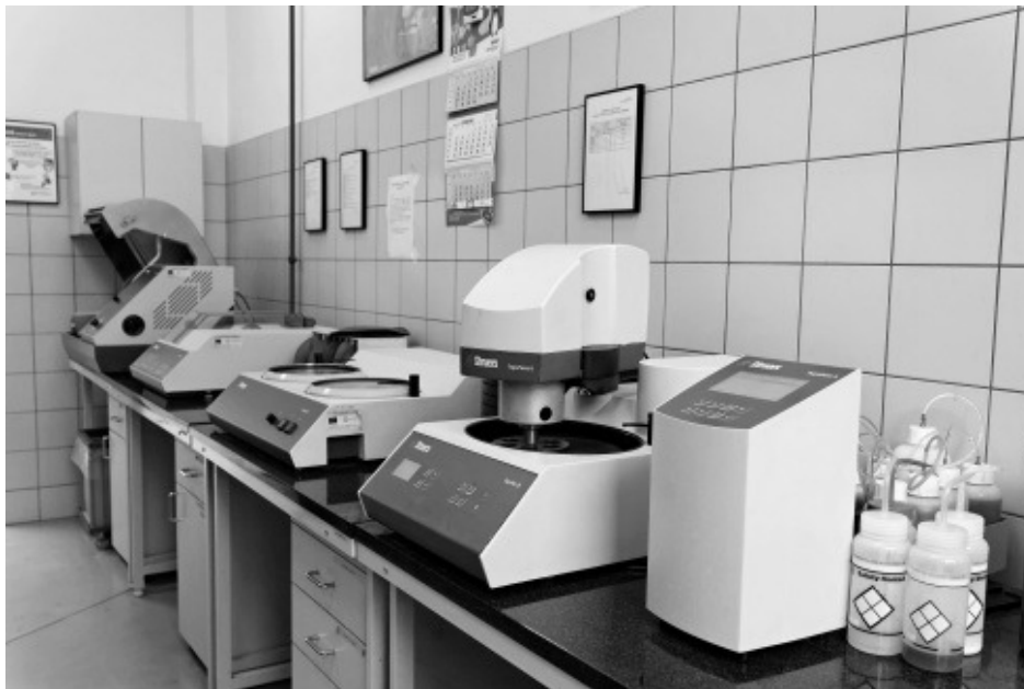
Figure 10 Metallography Laboratory for performing sample preparation (precision cutting, manual and automatic polishing and mounting) before the coating deposition process, also preparation after the process for microscopic observations. (Research and Development Laboratory for Aerospace Materials, 2014).
