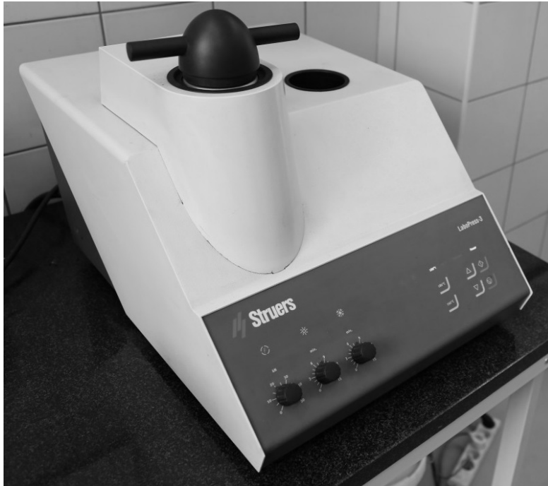
Figure 14. Fully automatic mounting press for hot mounting Struers LaboPress-3 (Research and Development Laboratory for Aerospace Materials, 2014).
