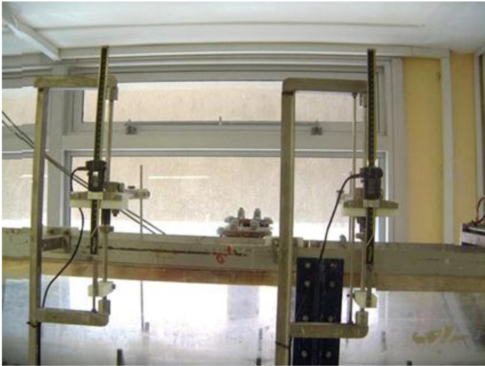
Figure D.2a Two Mitutoyo digital depth gauges mounted on the flume at 5 m and 6 m from the entrance
