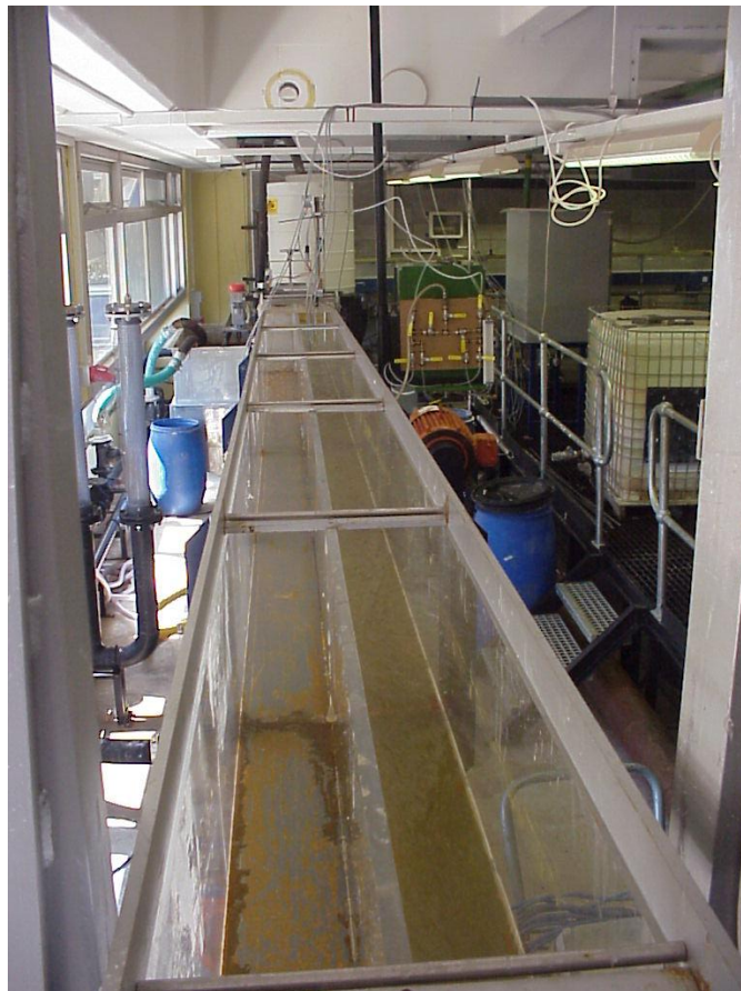
Figure D.1b Flume with partition fitted to form a 150 mm wide rectangular flume.
