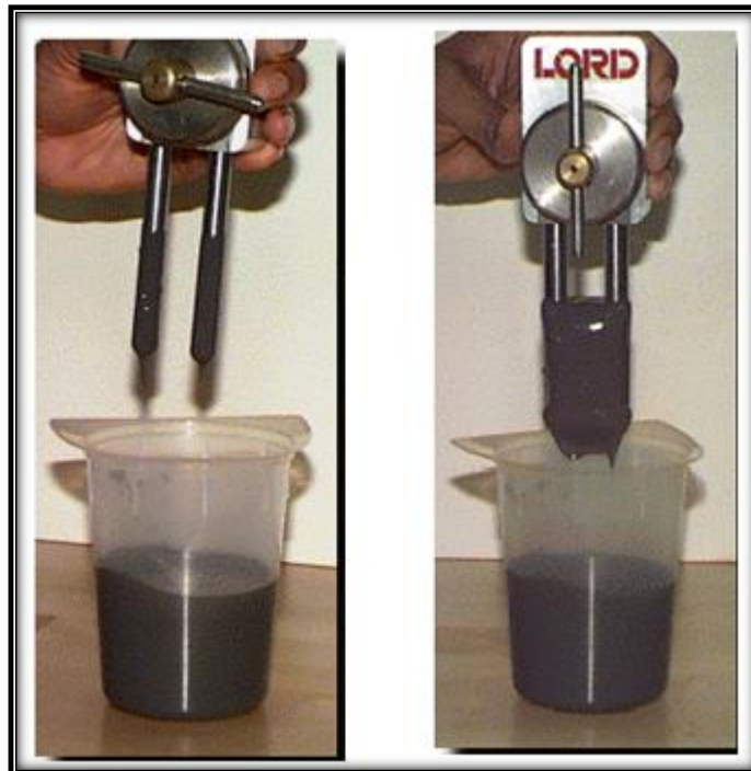
Figure1.18: The MR Fluid is liquid on the left, and as a solid in magnetic field on the right[2001 SMA/MEMS Research Group]
