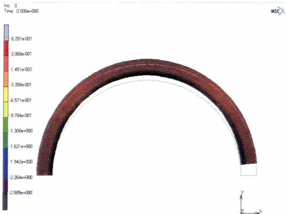
Figure 4.22: Contour plot of the actuator force in the X- direction at 0.31 thickness ratio
