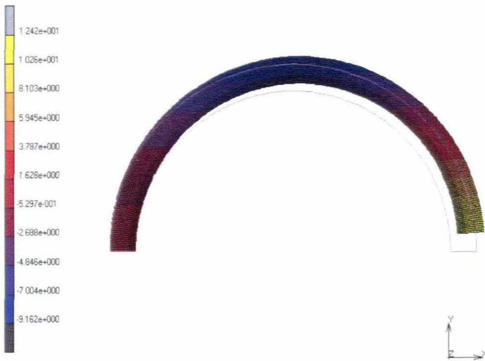
Figure 7.8: First Mode shape for a 0.25mm Aluminium substrate
