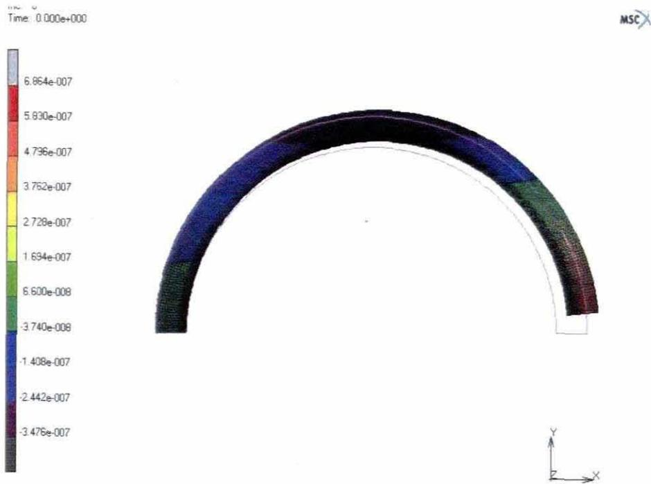
Figure 4.21: Contour plot of displacement in the X-direction, at 0.31 substrate/PZT thickness ratio
