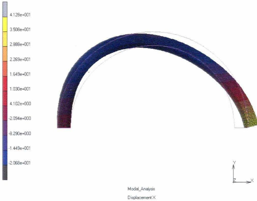
Figure 7.10: The third mode shape for a 0.25mm Aluminium substrate
