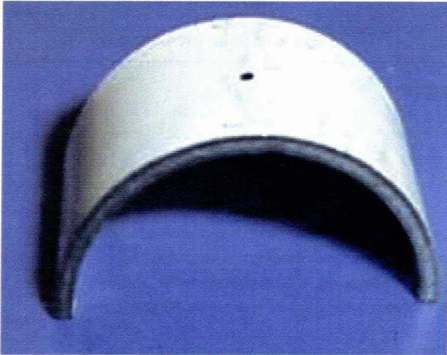
Figure 5.1: C-shape piezoceramic ring
