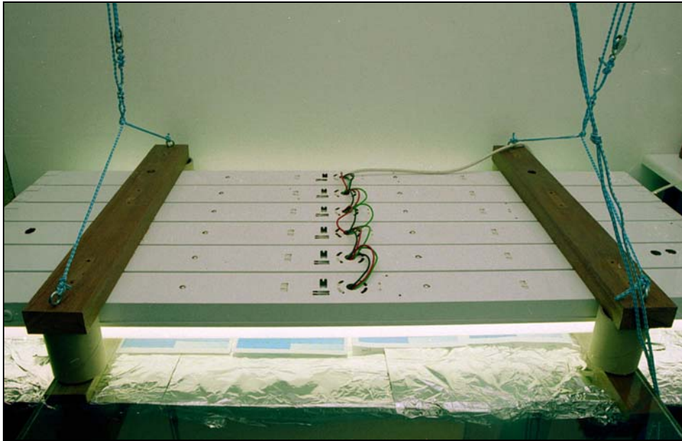
Figure 3.1. Accelerated fading exposure apparatus.
