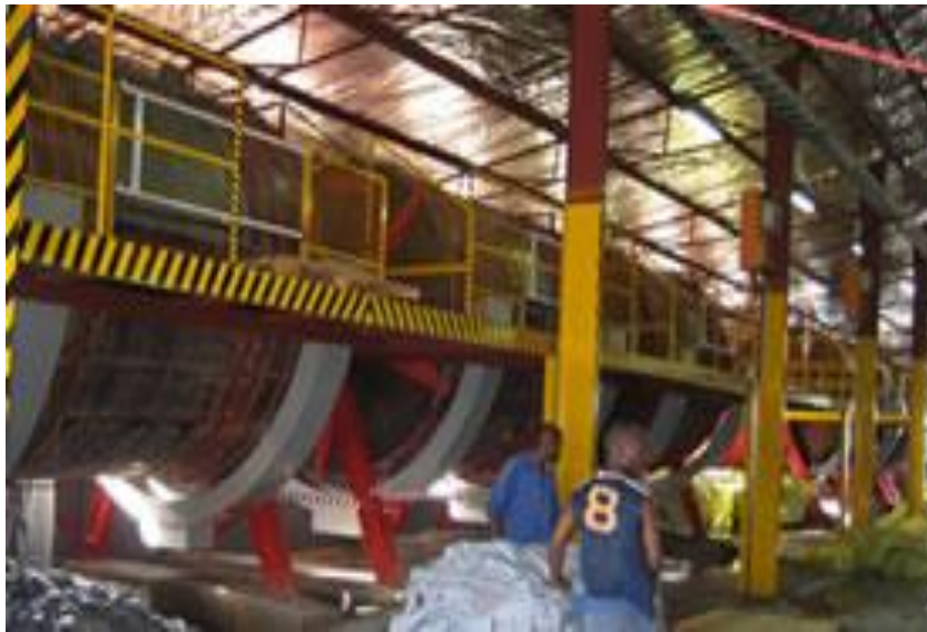
Figure.2.3: Chromium tanning drum (Source: Tannery industries of Botswana, 2013)
