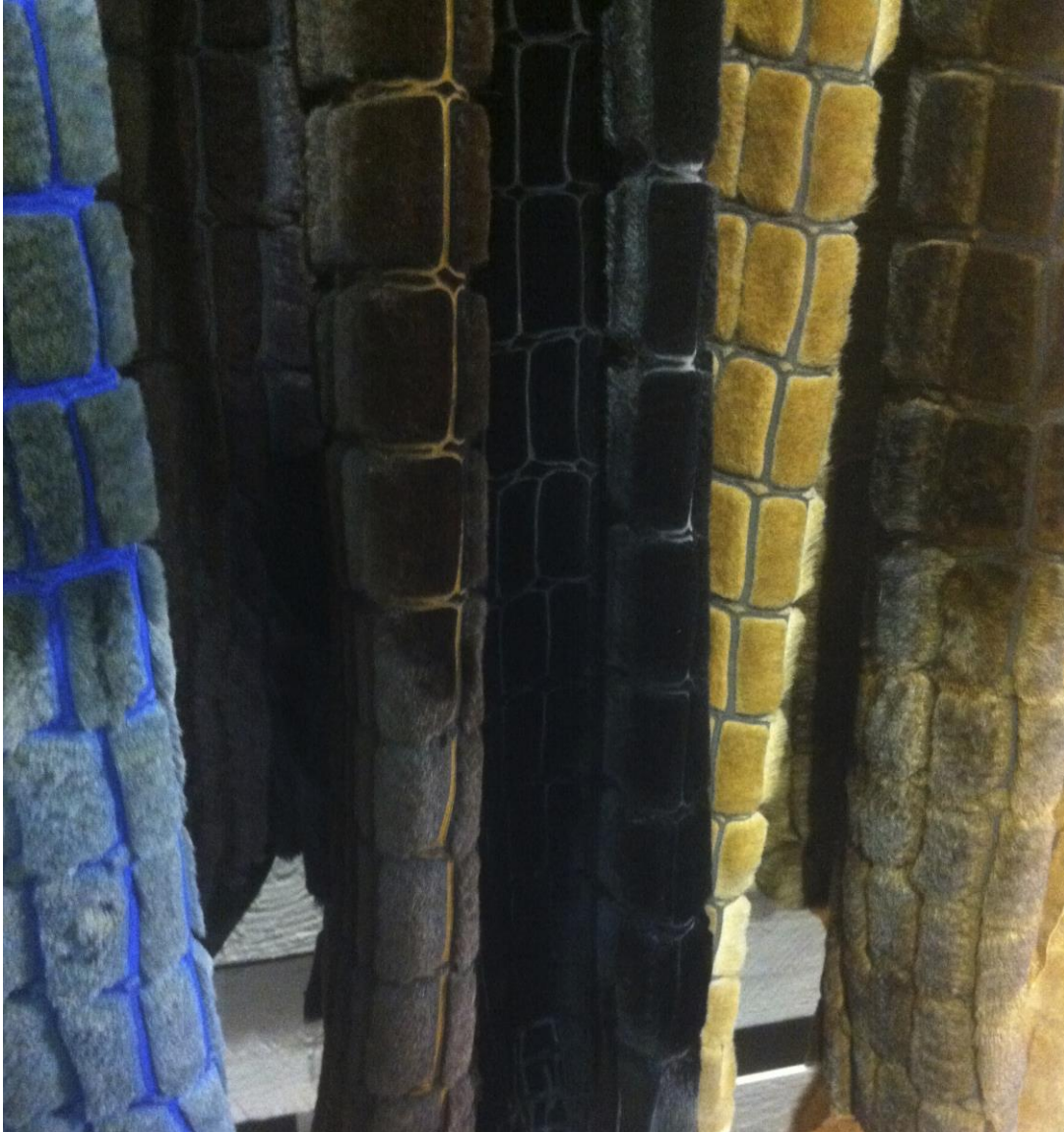
Figure 7.56: Hair on leather laser-cut pattern after dyeing (Source: Author's own, 2014)
