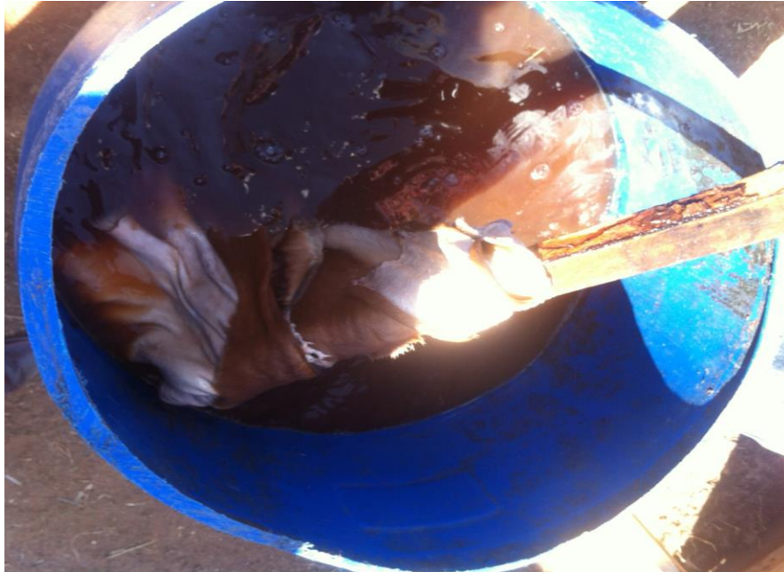
Figure 7.69: Kudu hide being stirred to ensure that the vegetable tannin is mixed (Source: Author's own, 2014)
