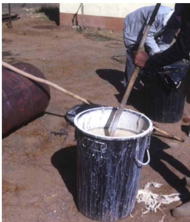
Figure 7.65: The liming process to remove hair from hides/skins (Source: Author's own, 2014)
