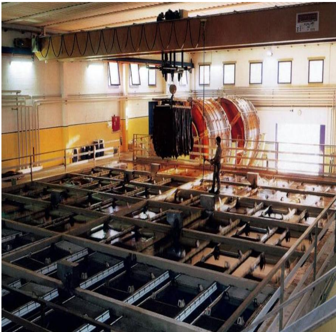
Figure 7.7 Modern tanning vats sunken to the surface with a drying rack suspended above (Source: Author's own)
