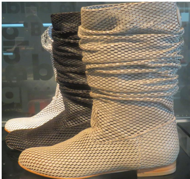
Figure 7.53: Laser-cut leather which used to make high-end footwear (Source: Author's own, 2013)
