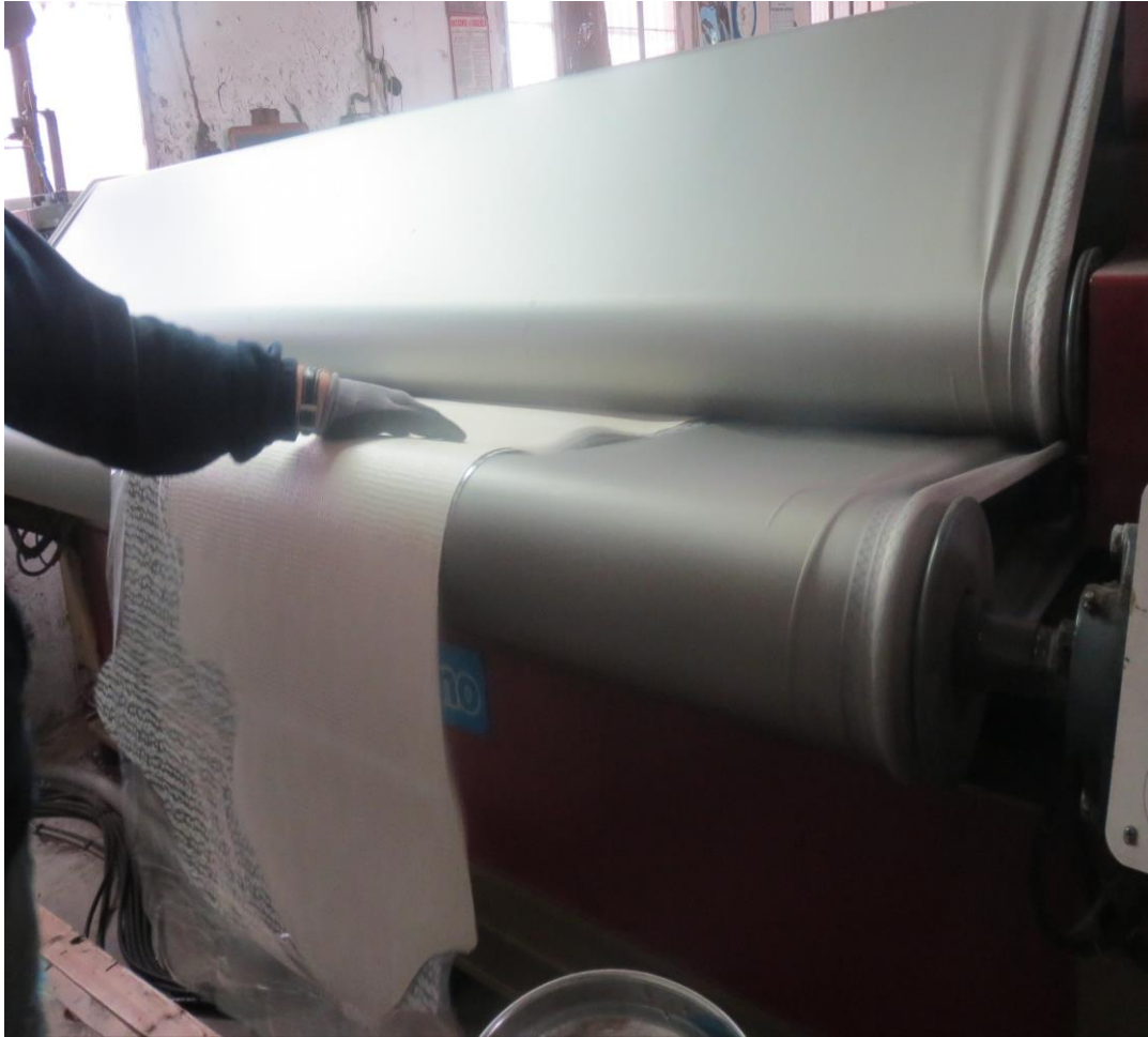
Figure 7.22: Pressing machine helps gives texture onto smooth surfaced leathers (Source: Author's own, 2014)
