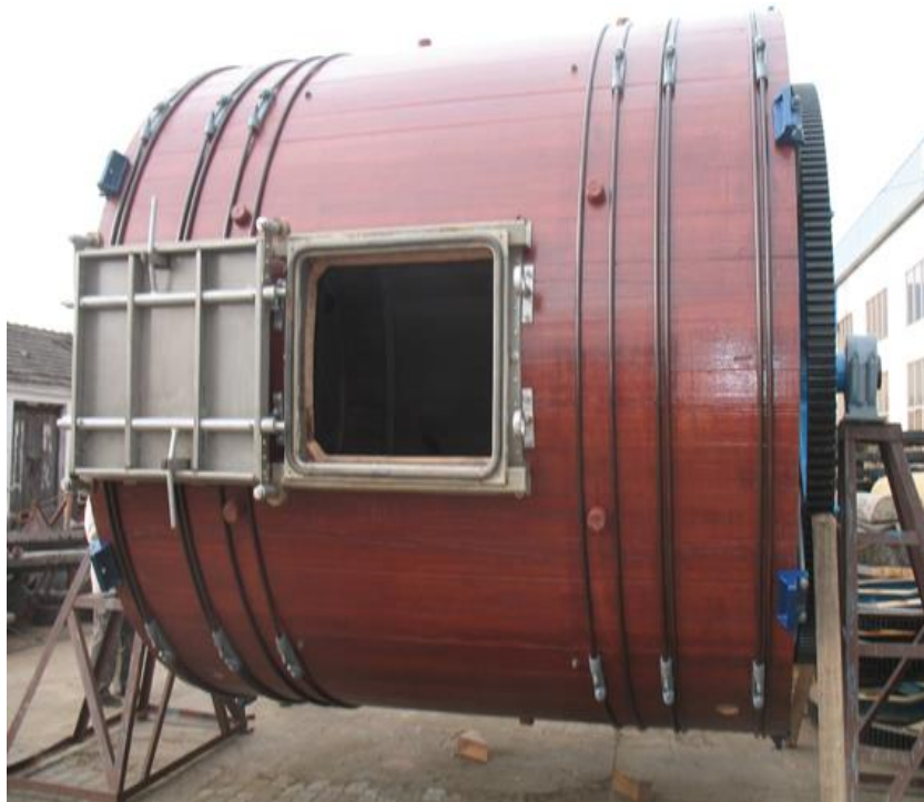
Figure 2.8: Modern wooden tanning, liming and dyeing drum with larger capacity (Source: Google images, 2013)
