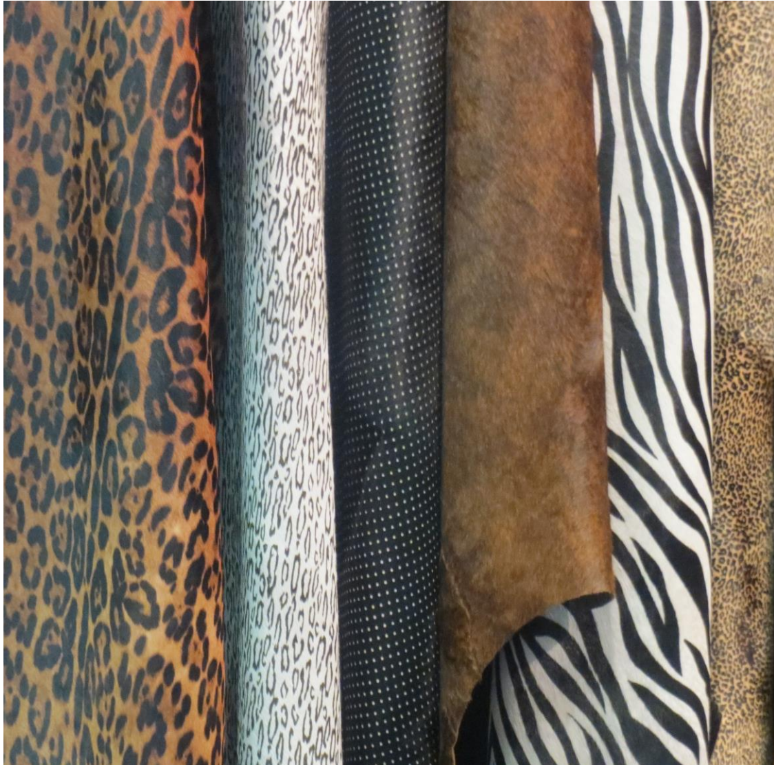
Figure 7.32: Hair on cow hides printed using a digital printer (Source: Author's own, 2014)
