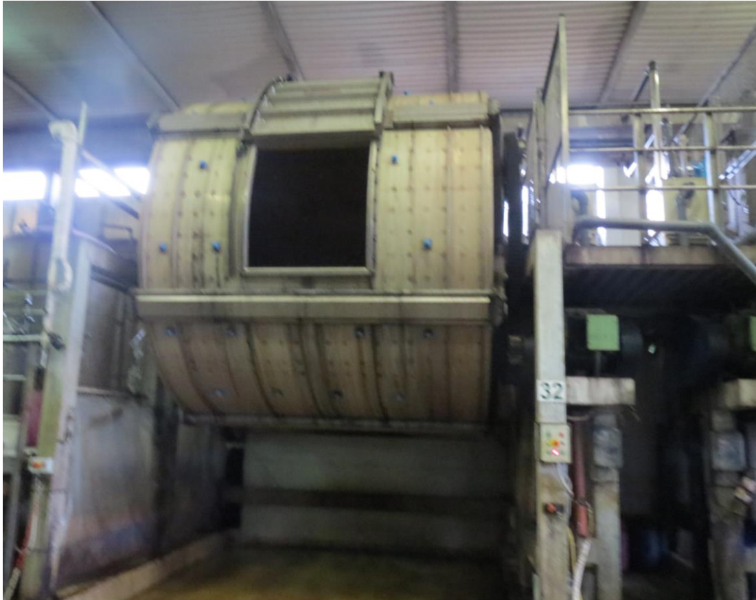
Figure 7.9: Leather tanning drum in front and tanning vats at the back of the drum (Source: Author's own, 2013)
