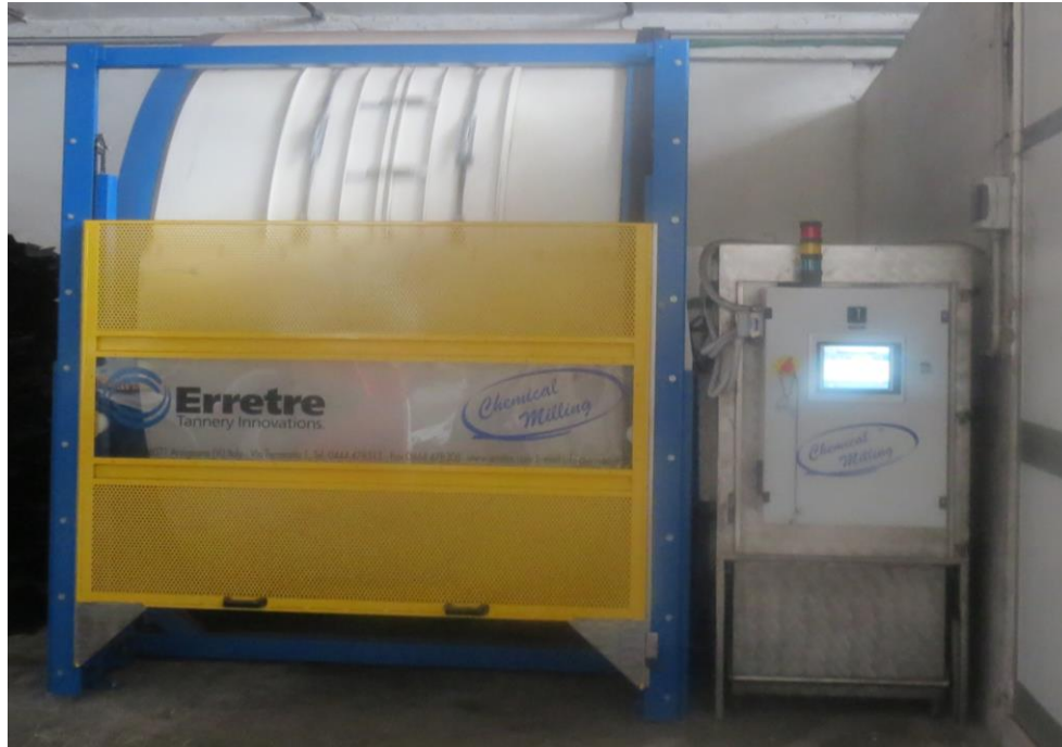
Figure 8.12: Semi-automated tanning drum (Source: Author's own, 2014)
