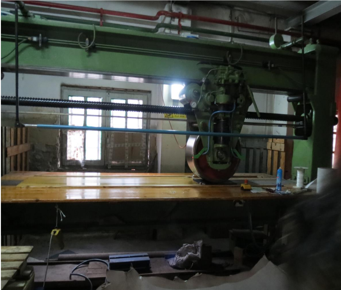
Figure 7.23: Ironing machine to get rid of moisture and to give leather the shiny effect (Source: Author's own, 2014)
