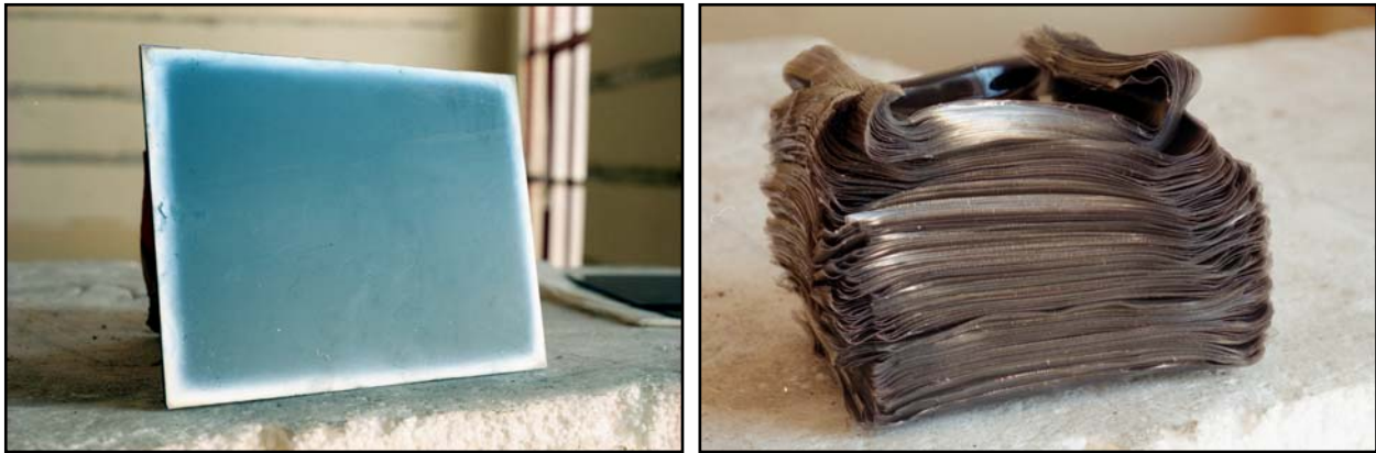
Figure 2.10 Silver mirroring (left) and negative curling and sticking (right)
