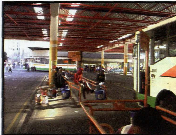
Figure 7.5: Seating at the Cape Town bus terminus is not suitable for SNPs because of the height and design.
