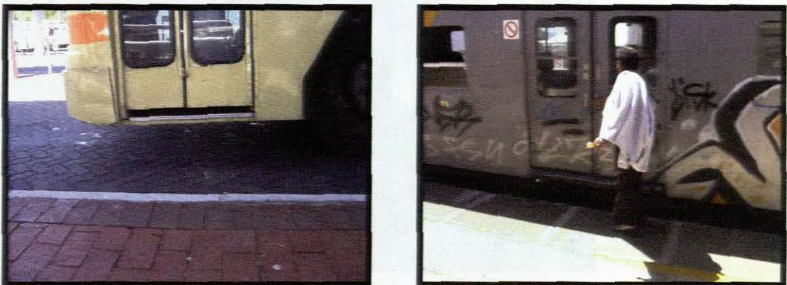
Figure 4.24: Bus and train – no level access present
