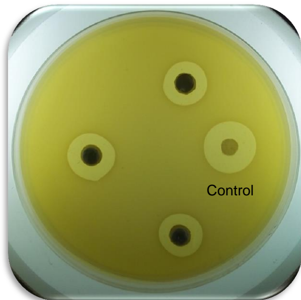
Figure 3.8: Antimicrobial activity of a preparation of treated \text{TiO}_2 nano-composite composite with 10% (m/m) benzalkonium chloride against E. coli . It is evident that the preparation possesses antimicrobial activity.
