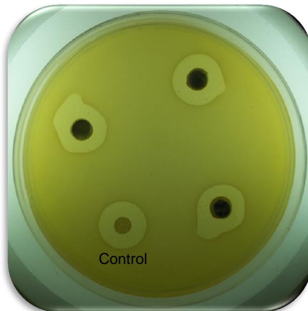
Figure 3.4: Antimicrobial activity of a preparation of treated \text{TiO}_2 nano-composite composite with 10% (m/m) chlorhexagluconate tested against E. faecalis . It is evident that the preparation possesses antimicrobial activity.
