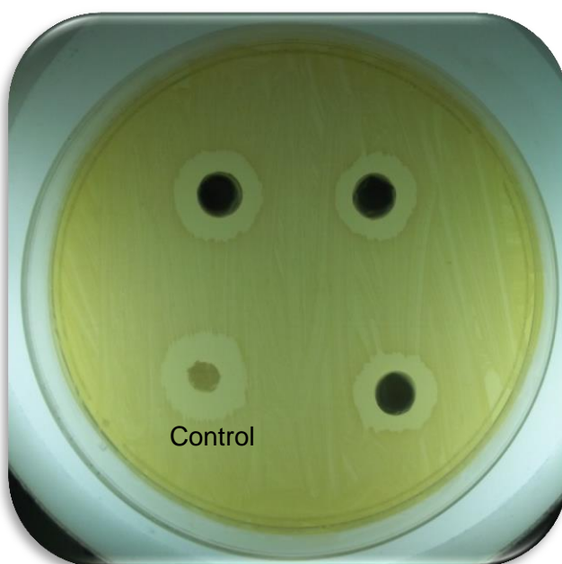
Figure 3.12: Antimicrobial activity of a preparation of treated \text{TiO}_2 nano-composite composite with 10% (m/m) benzalkonium chloride tested against S. mutans . It is evident that the preparation possesses antimicrobial activity.
