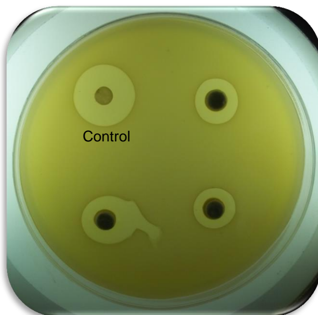
Figure 3.11: Antimicrobial activity of a preparation of treated \text{TiO}_2 nano-composite composite with 10% (m/m) benzalkonium chloride tested against S. aureus . It is evident that the preparation possesses antimicrobial activity.
