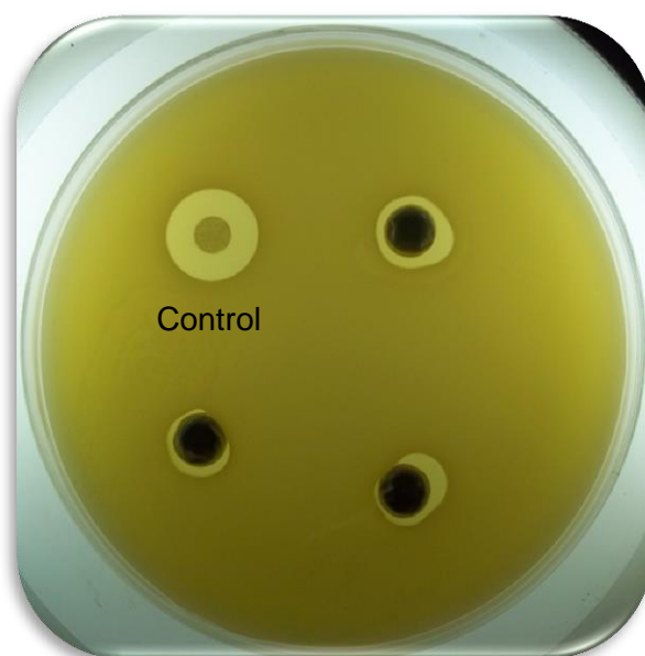
Figure 3.14: Antimicrobial activity of a preparation of treated TiO 2 nano-composite composite with 5% (m/m) benzalkonium chloride tested against S. aureus . It is evident that the preparation possesses antimicrobial activity.
