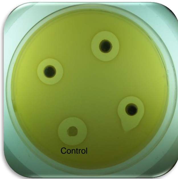
Figure 3.9: Antimicrobial activity of a preparation of treated \text{TiO}_2 nano-composite composite with 10% (m/m) benzalkonium chloride tested against E. faecalis . It is evident that the preparation possesses antimicrobial activity.
