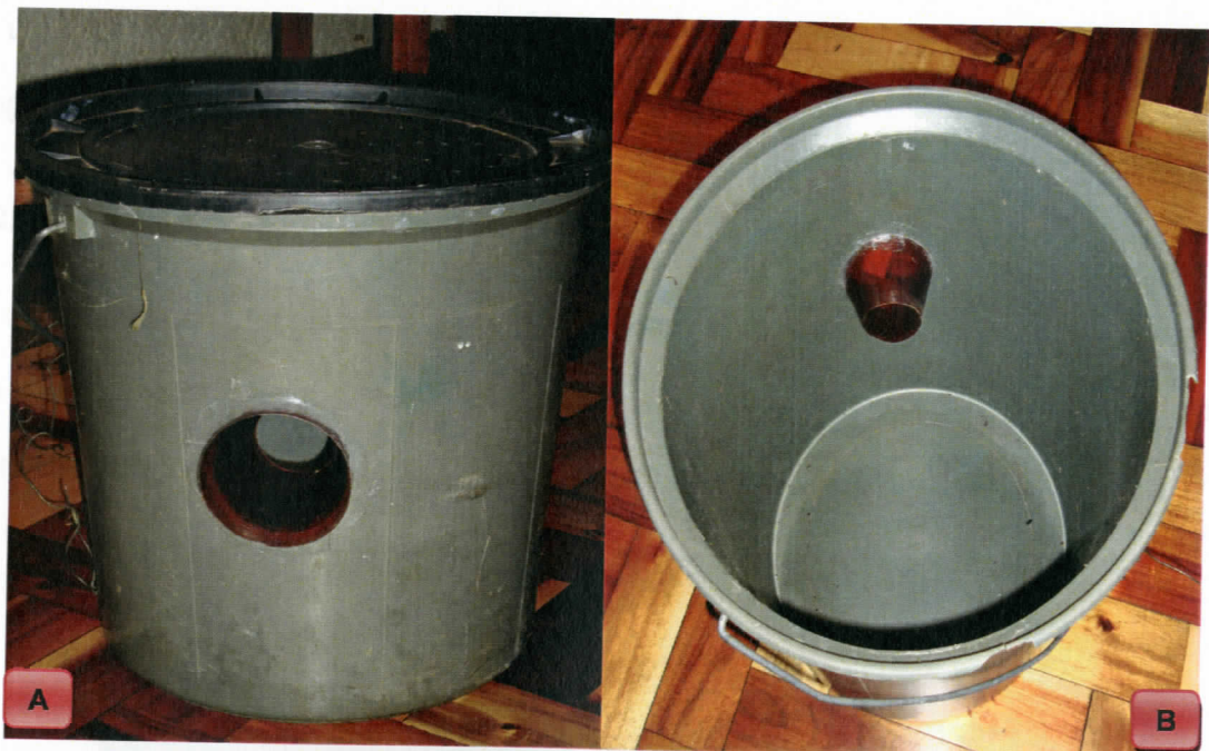
Figure 2.2: Home - made bucket trap. The exterior of the trap is shown in A, whilst B depicts the interior
