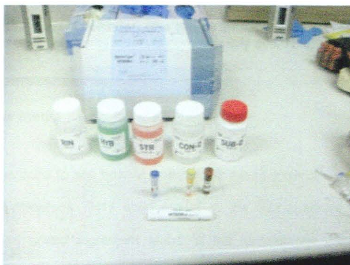
Figure 2.12 Components of the GenoType®MTBDRs/ kit, which are used for testing the fluoroquinolones, aminoglycosides and ethambutol.
