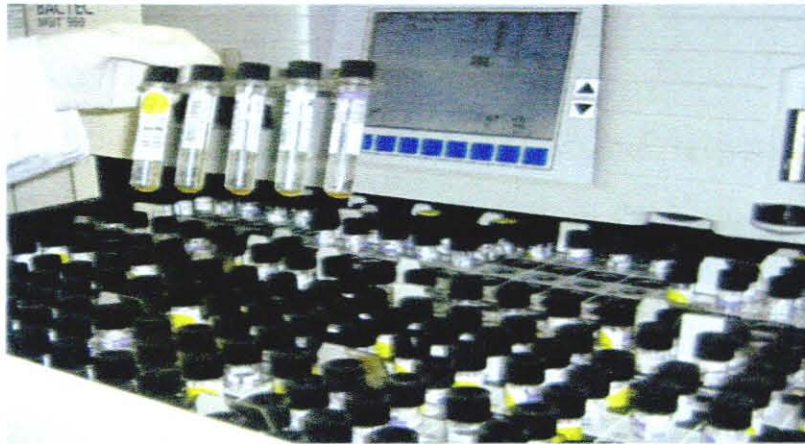
Figure 2.10 Loading of a MGIT SIRE™ carrier set, consisting of a sample growth control and four MGIT SIRE™ tubes, each containing a different antibiotic, streptomycin, isoniazid, rifampicin and ethambutol.
