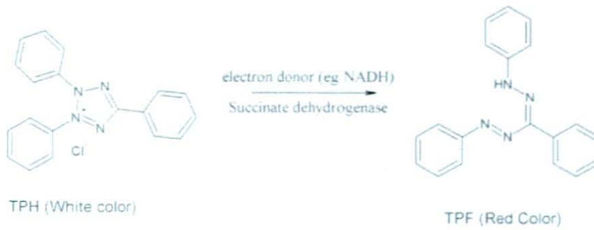
Figure 3.3 Chemical structure of TTC , which is a redox indicator. The white compound is enzymatically reduced to red TPF (1,3,5-triphenylformazan) in living tissues due to the activity of various dehydrogenases during oxidation of organic compounds (Wikipedia, 2010).
