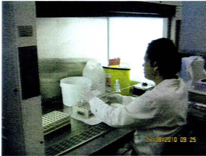
Figure 2.1 Biological safety cabinet and protective clothing such as coats and gloves were worn to prevent contamination when handling potentially pathogenic specimens. Also note other safety measures such as a sharps container, a container to discard the supernatant of the specimens and a bucket containing 5% phenol solution for other waste items such as orange sticks (Pathcare).
