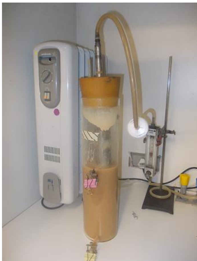
Figure 5.3: Photograph showing Streptomyces sp. strain BSII growing in an airlift reactor. On the right (in the rear) is a flow meter device for measuring air flow rate as it was pumped into the reactor.
