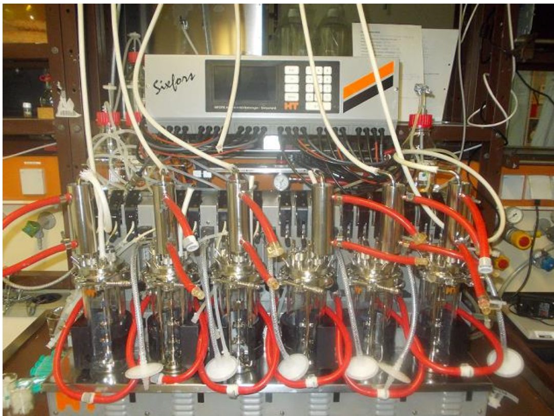
Figure 5.4: Photograph of the parallel Sixfors bioreactor system used. The system comprises six independent fermentation units that can be independently controlled for pH, temperature, stirrer speed and antifoam activity.
