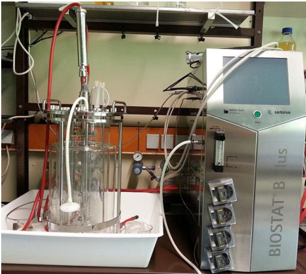
Figure 5.5: Photograph showing a Sartorius Biostat B fermentor. On the left is the stirred tank fermentor and its associated attachments, and on the right is the control unit.
